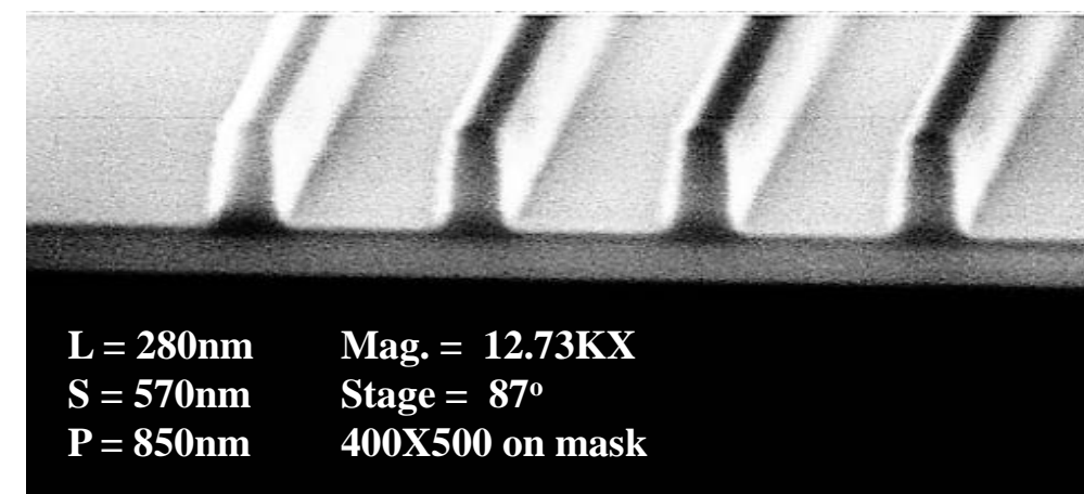
Figure 6. Resist Patterning Through Annular Illumination.
