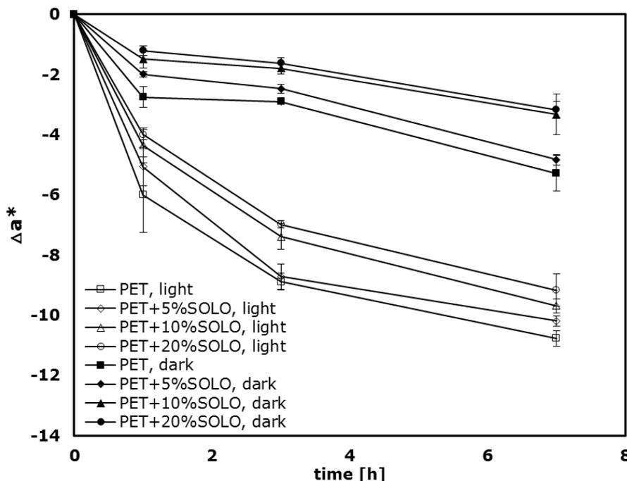
Figure 3 Changes in redness ( $\Delta a^* = a^*_t - a^*_{t=0}$ ) of ham slices packaged in neat PET and active films at different percentage of oxygen scavenger, during 7 days storage at  $4 \pm 1^\circ\text{C}$ . Color of the symbols indicate whether the samples were stored in dark (black) or illuminated conditions. Mean value  $\pm$  standard deviation.
