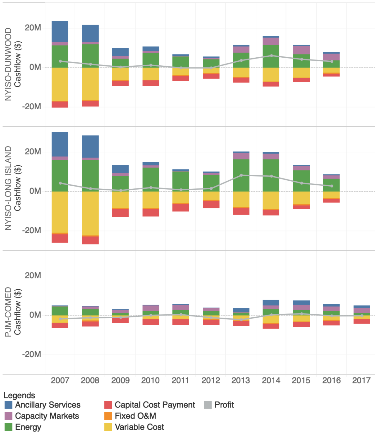
FIGURE 7: Cash flow of 50MW Natural Gas Combustion Turbine power plant operating in PJM-COMED, NYISO-Long Island, NYISO-Dunwood. It shows the revenue from capacity, energy and ancillary services markets as positive values, and the fixed O&M cost, variable cost and capital cost payment as negative values and the profit in each year. It shows that in each of the market the
