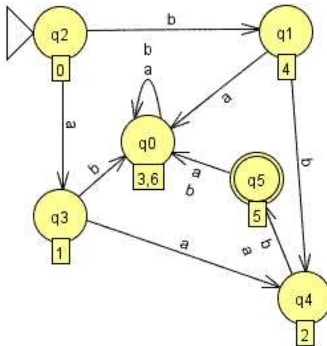
Figure 21: The minimized DFA produced by JFLAP.
