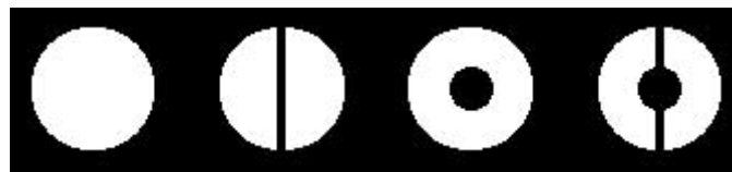
Figure 3.2. Clear, "Half-Moon", Cassegrain, and Hinged Apertures
