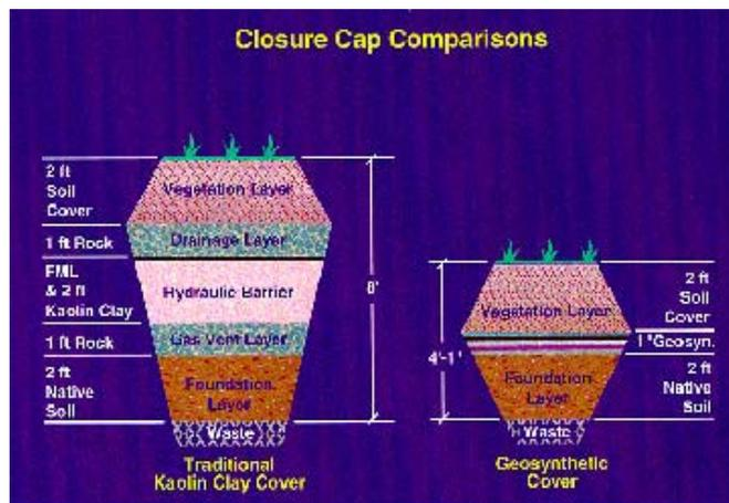
Figure 1: Visual diagram of the layers used in traditional and geosynthetic capping [2].
