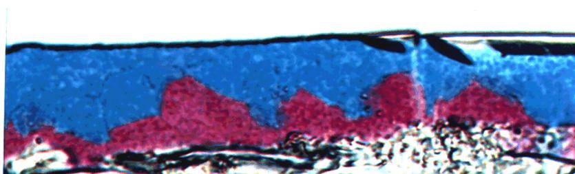
Figure 5: Image Cross Section of Multi Layer Blue 100% Coverage Sample Patch
