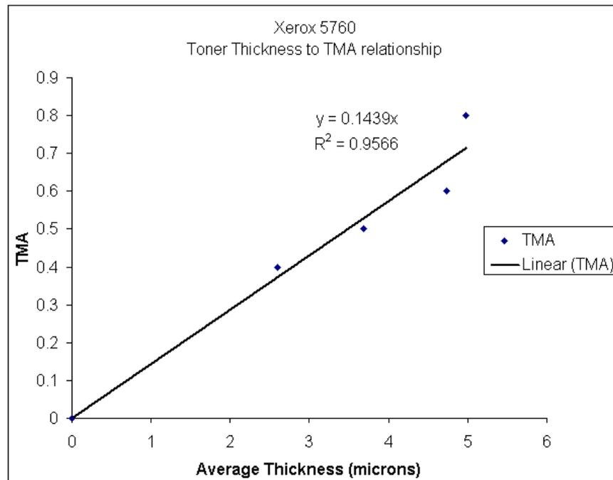
Figure 7: Linear Relationship between toner thickness and toner mass per unit area (TMA)
