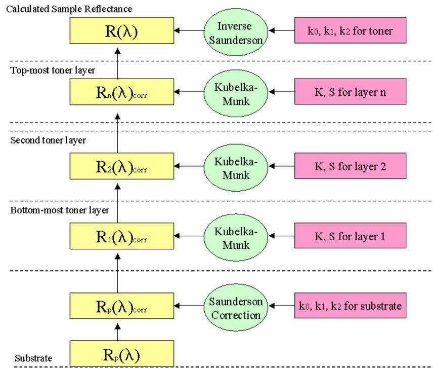
Figure 3: Flowchart illustrating the method for modeling the reflectance of a multi-layer image
