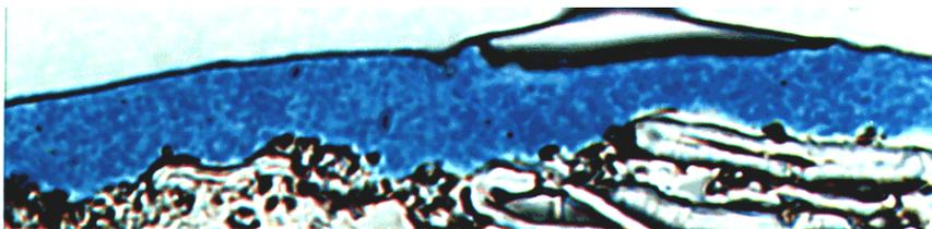
Figure 4: Image Cross Section of Single Layer Cyan 100% Coverage Sample Patch
