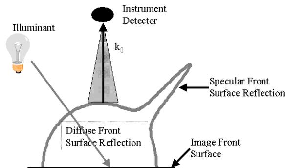
Figure 1: Illustration of the Correction Parameters  $k_0$  and  $k_1$
