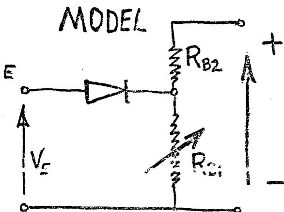
When a positive potential at point E forward biases D1 an output will result. Refer to oscillator circuit ( figure 3 ). Each capacitor, C1 thru C3, when connected ( seperately ) forms a RC time constant which determines the minimum time to reach the forward bias potential needed at point E to obtain an output. In this manner the audio frequency region is scanned.
