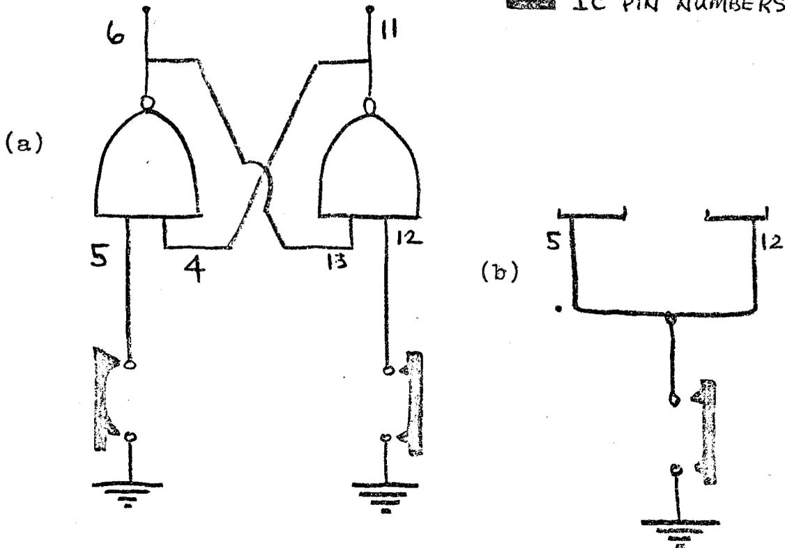
Circuit a is a basic flip flop, obtained from the cross coupling of two nand gates.
