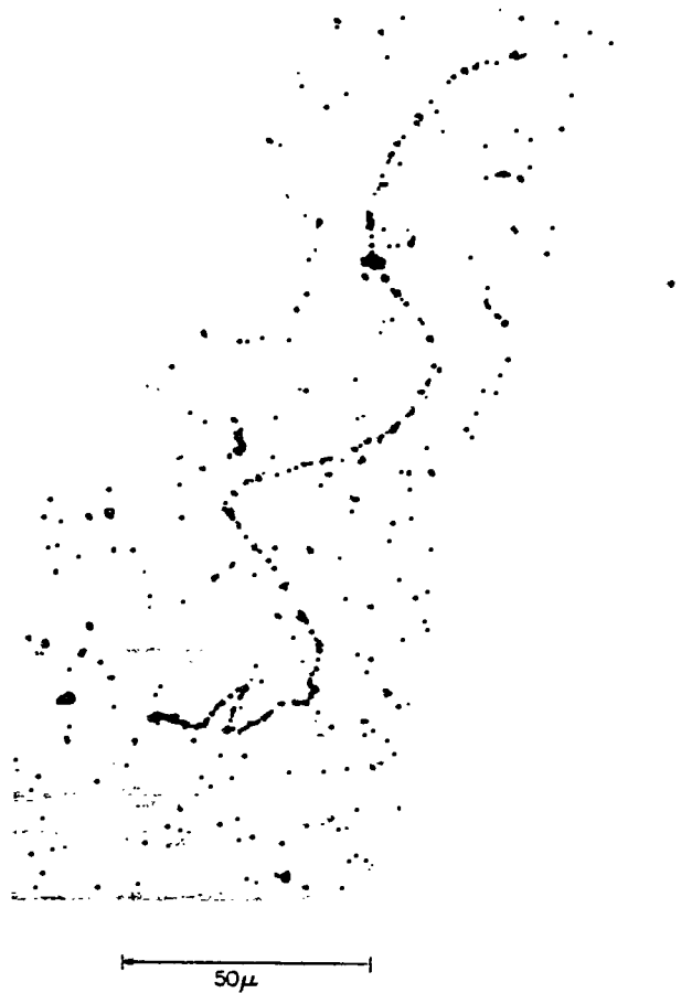
Figure 4.3. Photomicrograph of an electron track as seen in a nuclear track emulsion.
