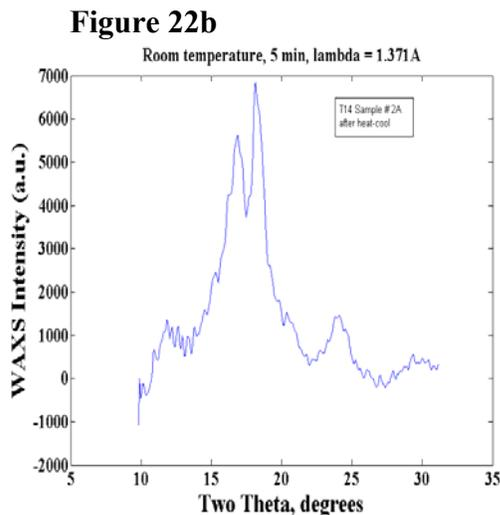
**Figure 22b** In the composite film that gave α-phase X-ray diffraction spectrum shown in Figure 22b. α-phase Poly[4(5)-VIm] was protonated with 15 mol% TFSI, dissolved in DMF. Cast from DMF at ambient temperature and dried at 100°C and annealed at 200°C
