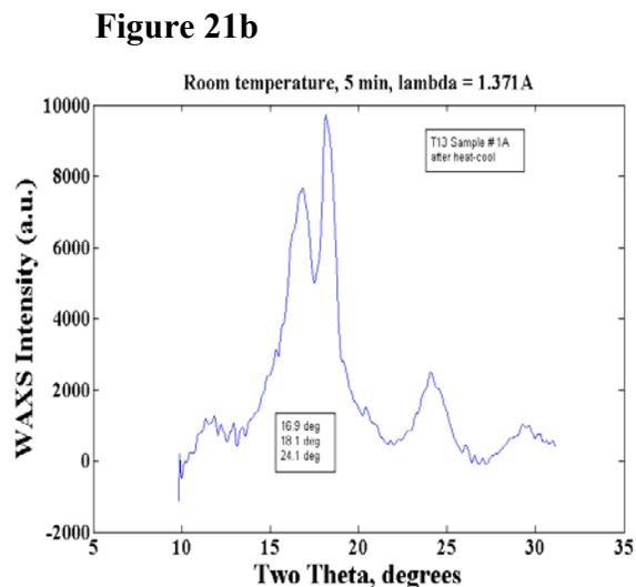
**Figure 21b**  $\alpha$ -phase PVF<sub>2</sub> cast from DMF at ambient temperature and dried at 100 °C and annealed at 200°C
