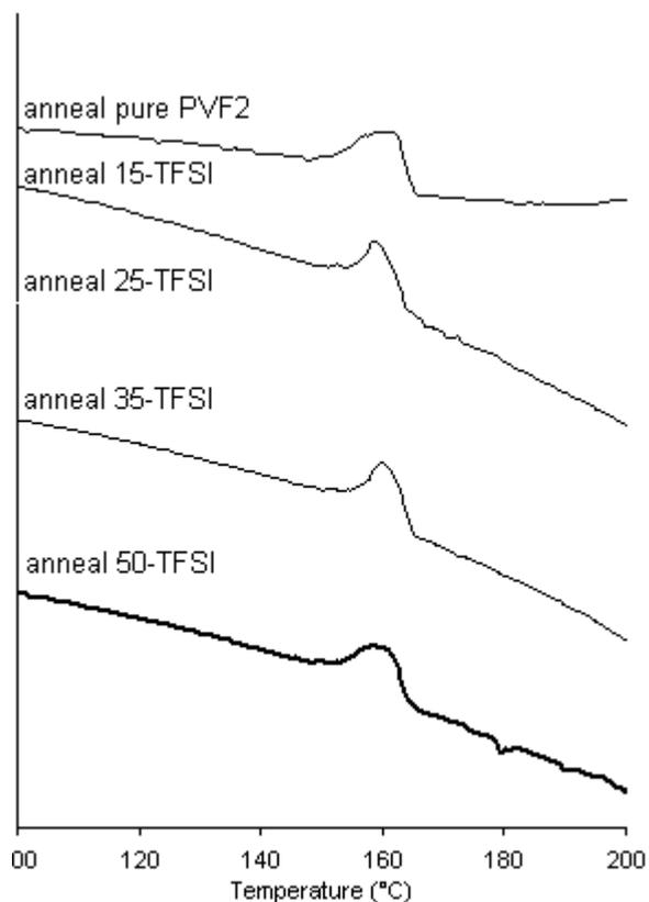
**Figure 29b** DSC thermograms for the 2<sup>nd</sup> heating scan of non-heated film of PVF<sub>2</sub> and the composites from DMAC
