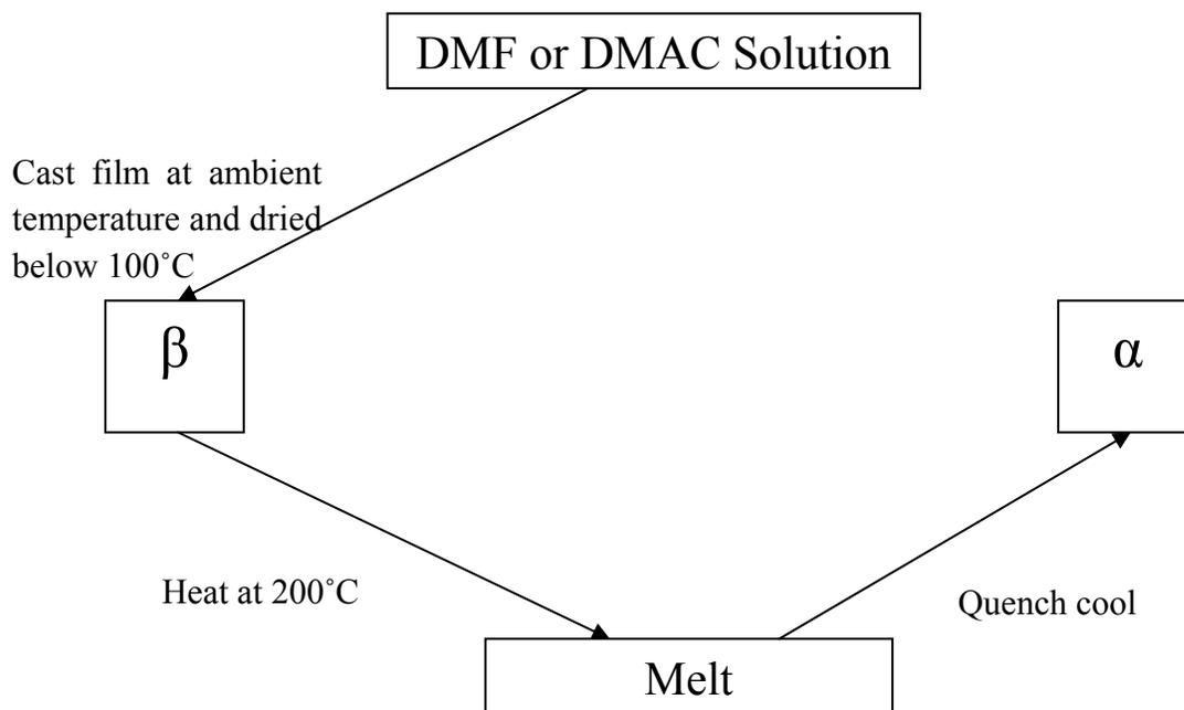
**Figure 27. Transformation between the two main phases of PVF<sub>2</sub>**
