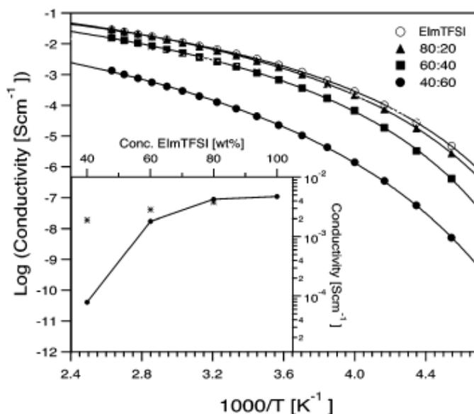
**Figure 14. Ionic conductivity of PVF<sub>2</sub>/EIm<sup>+</sup>TFSI composite membranes<sup>27</sup>**
