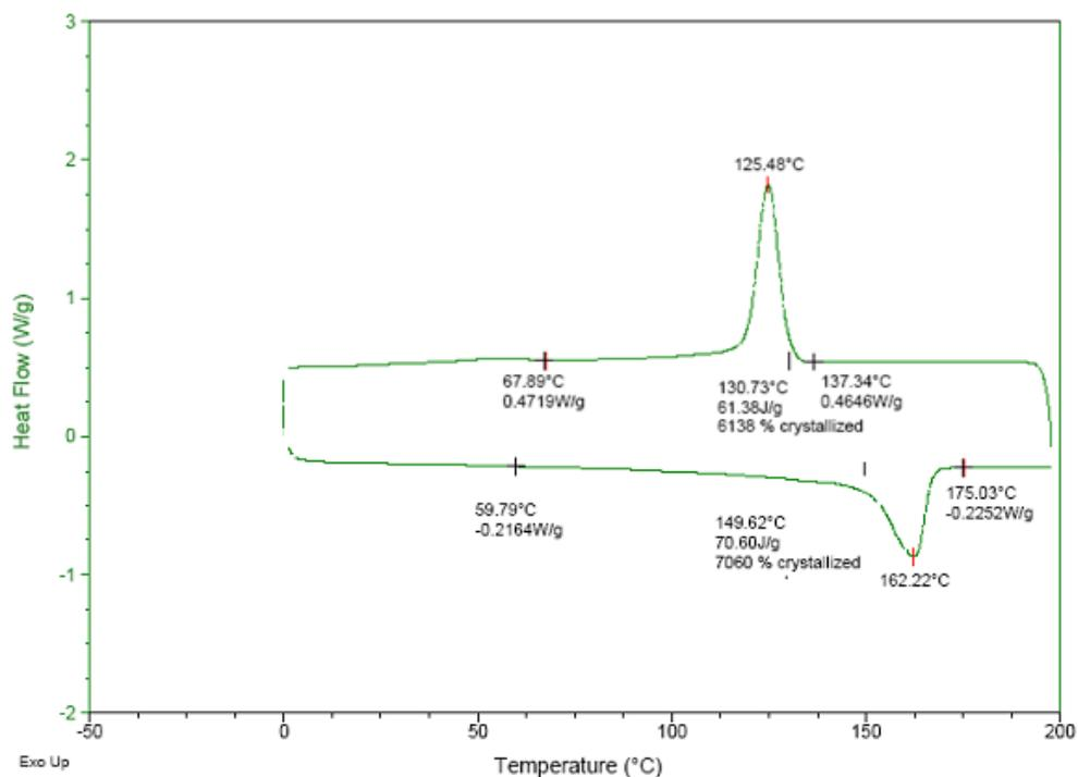
**Figure 28. Heating and cooling cycle scans in DSC of Kynar®301 PVF<sub>2</sub>**
