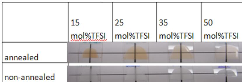
**Figure 20. PVF<sub>2</sub>/PVIm-Im<sup>+</sup>TFSI<sup>-</sup> composite films cast from DMAC**
