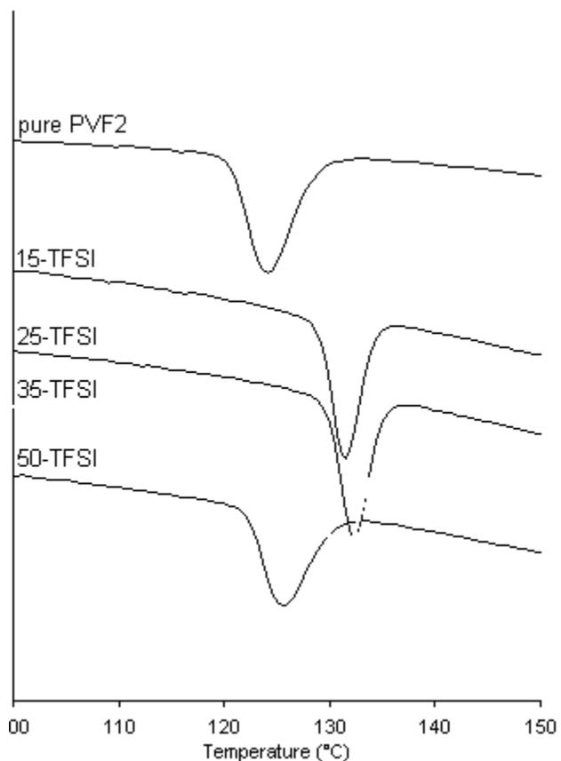
**Figure 34a** DSC thermograms for the cooling scan of non-heated film of PVF<sub>2</sub> and the composites from DMAC
