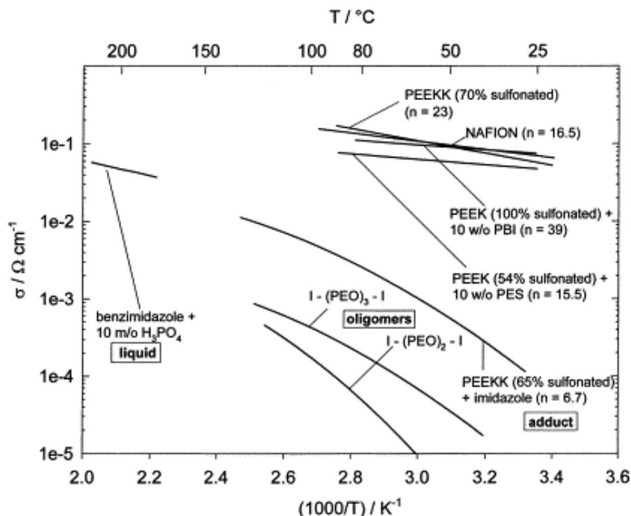
**Figure 4. Proton conductivity of different fully hydrated acidic polymers, the liquid benzimidazole/ $\text{H}_3\text{PO}_4$  system, and ethoxylated imidazole oligomers**<sup>10</sup>
