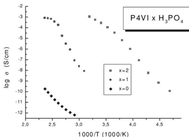
**Figure 12. Temperature dependence of DC conductivities of poly(4-vinylimidazole) and the poly(4-vinylimidazole)- $x$   $H_3PO_4$  blends**<sup>25</sup>
