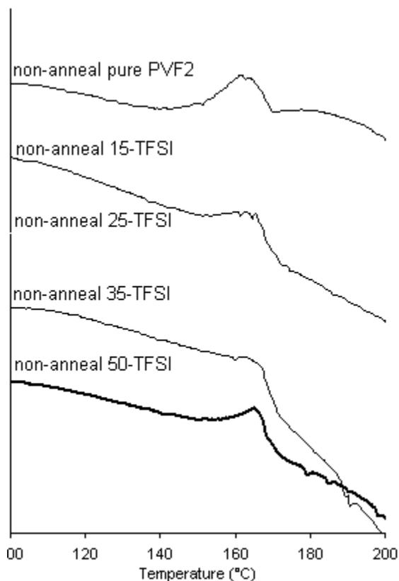
**Figure 29a** DSC thermograms for the 1<sup>st</sup> heating scan of non-heated film of PVF<sub>2</sub> and the composites from DMAC
