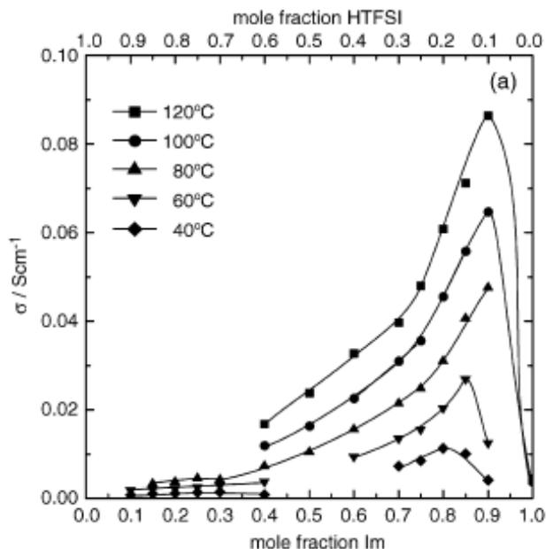
**Figure 15. Ionic conductivity as a function of the mole fraction of imidazole (Im) in Im/bis(trifluoromethanesulfonyl)imide (HTFSI) mixtures**<sup>29</sup>
