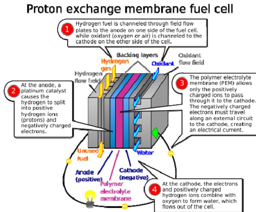
Figure 1. Illustration of a PEM fuel cell<sup>4</sup>
