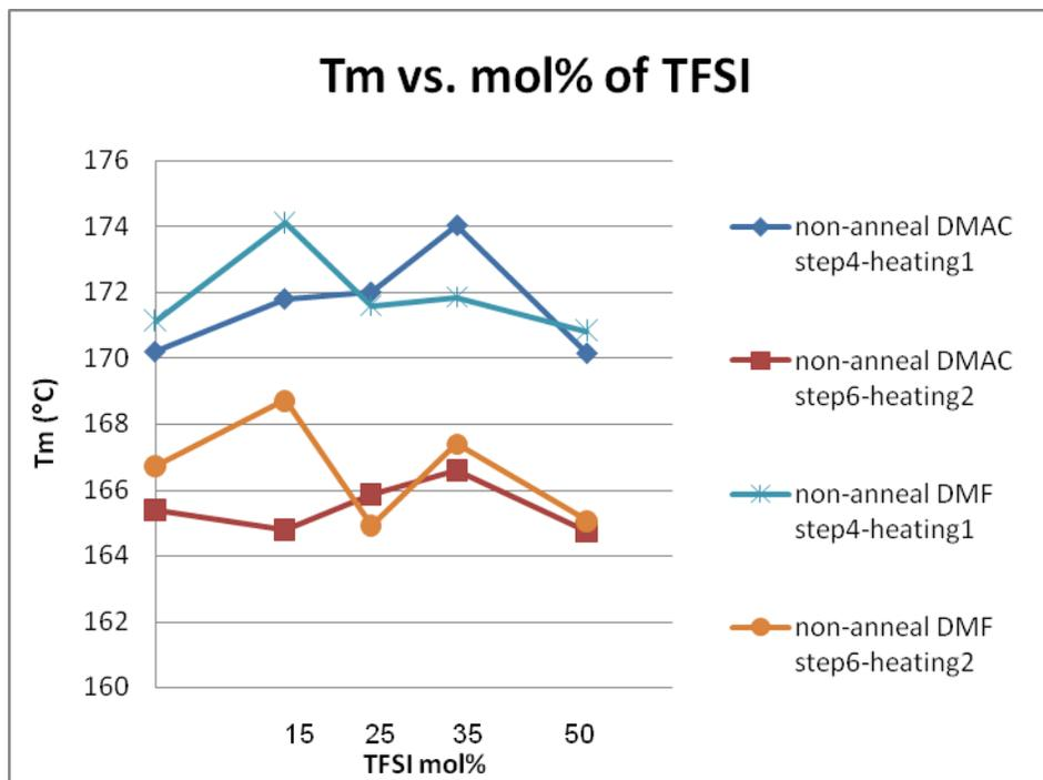
**Figure 33. Melting temperature of PVF<sub>2</sub>/poly[4(5)-VIm/VIm<sup>+</sup>TFSI] (4/1)<sub>v</sub> in DMF and DMAC**
