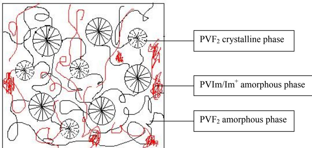
**Figure 37. Visualized microstructure of PVF<sub>2</sub>/poly[4(5)-VIm/VIm<sup>+</sup>TFSI] composites**
