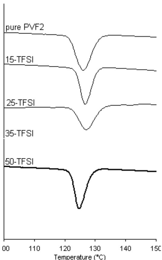
**Figure 34b** DSC thermograms for the cooling scan of non-heated film of PVF<sub>2</sub> and the composites from DMF
