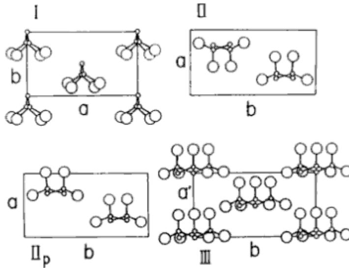
**Figure 6. Crystal structure of four crystalline modifications of PVF<sub>2</sub><sup>19</sup>**
