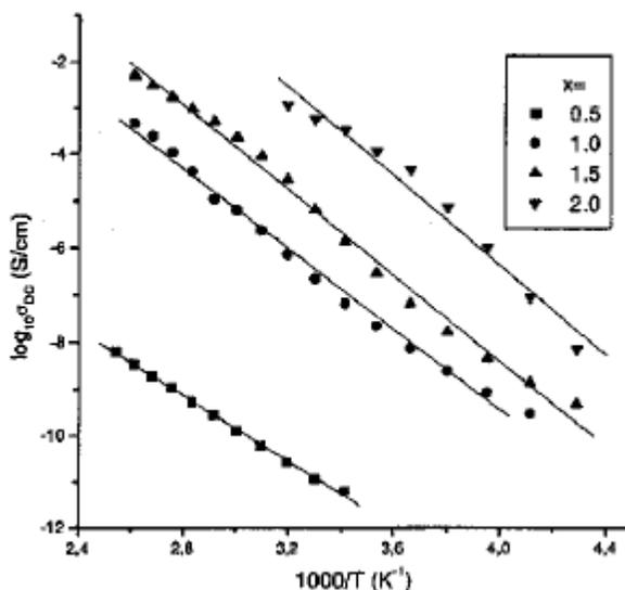
**Figure 11. Temperature dependence of DC conductivity of poly[4(5)-vinylimidazole] blended with  $\text{H}_3\text{PO}_4$  at various molar concentration ratios,  $X$ .<sup>24</sup>**
