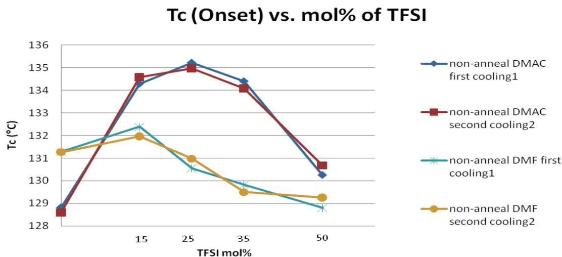
**Figure 35. Onset  $T_c$  of PVF<sub>2</sub>/poly[4(5)-VIm/VIm<sup>+</sup>TFSI] (4/1)v in DMF and DMAC**
