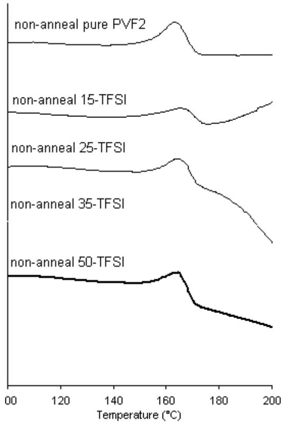
**Figure 30a** DSC thermograms for the 1<sup>st</sup> heating scan of non-heated film of PVF<sub>2</sub> and the composites from DMF
