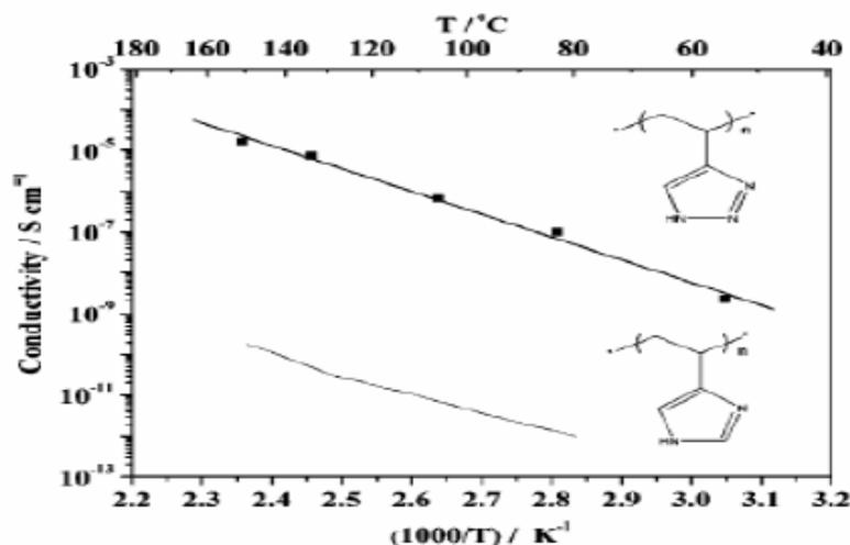
**Figure 13. Proton conductivity of poly(4-vinyl-1H-1,2,3-triazole) and poly(4-vinylimidazole)<sup>26</sup>**
