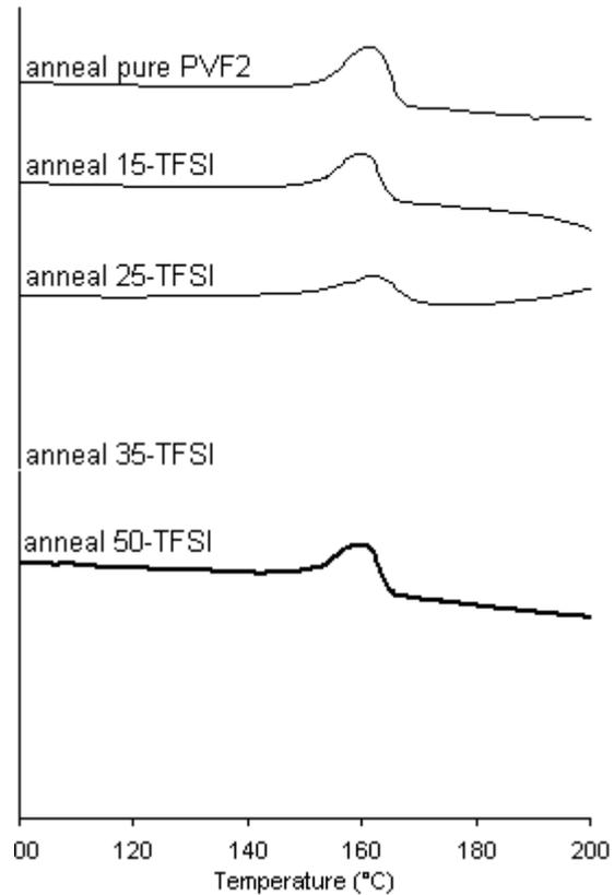
**Figure 30b** DSC thermograms for the 2<sup>nd</sup> heating scan of non-heated film of PVF<sub>2</sub> and the composites from DMF
