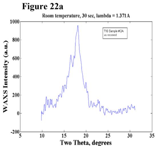
**Figure 22a** In the composite film that gave β-phase X-ray diffraction spectrum shown in Figure 22a. Poly[4(5)-VIm] was protonated with 15 mol% TFSI, dissolved in DMF. Cast from DMF at ambient temperature and dried at 100°C
