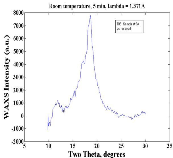
**Figure 26a**  $\beta$ -phase Poly[4(5)-VIm] was protonated with 35 mol% TFSI, dissolved in DMAC. Cast from DMF at ambient temperature and dried at 100°C
