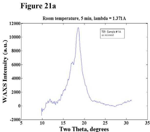
**Figure 21a** X-ray diffraction spectrum of  $\beta$ -phase PVF<sub>2</sub> cast from DMF at ambient temperature and dried at 100°C
