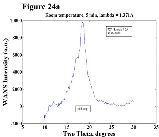
**Figure 24a**  $\beta$ -phase PVF<sub>2</sub> cast from DMAC at ambient temperature and dried at 100°C
