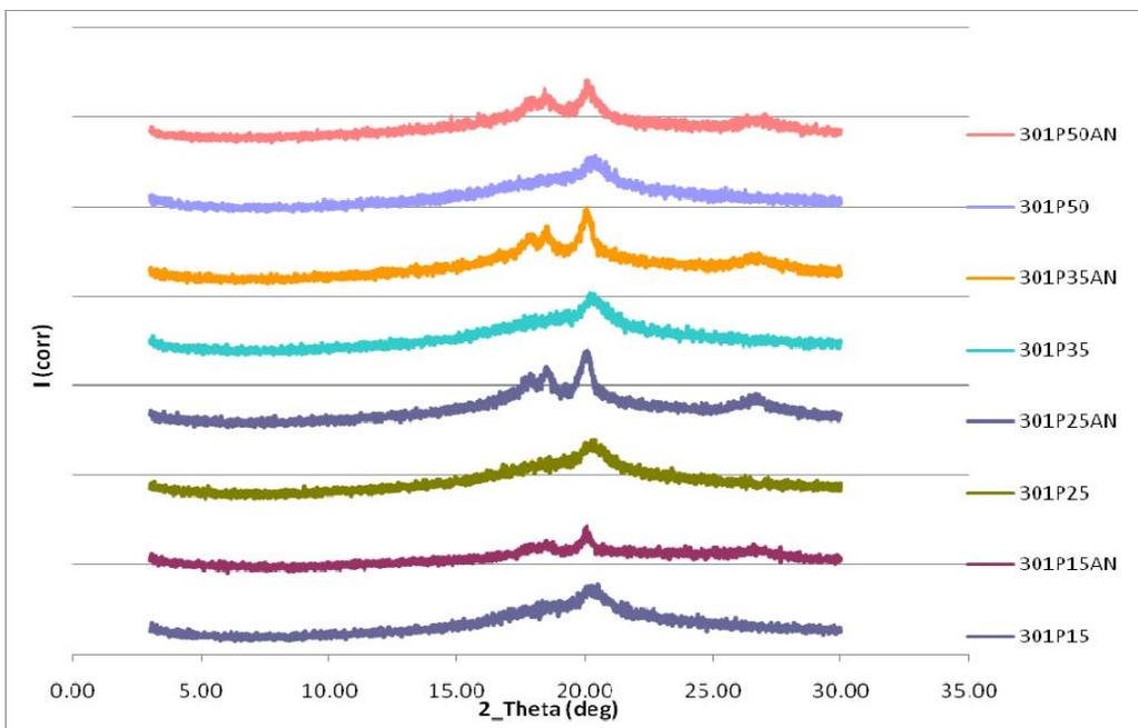
**Figure 19. X-ray diffraction traces (spectra) of PVF<sub>2</sub>/PVIm-Im<sup>+</sup> composite films cast from DMAC**
