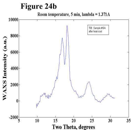
**Figure 24b**  $\alpha$ -phase PVF<sub>2</sub> cast from DMAC at ambient temperature and dried at 100°C and annealed at 200°C
