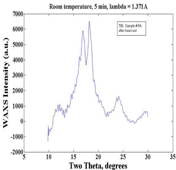
**Figure 26b**  $\alpha$ -phase Poly[4(5)-VIm] was protonated with 35 mol% TFSI, dissolved in DMAC. Cast from DMF at ambient temperature and dried at 100°C and annealed at 200°C
