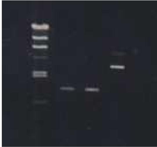
**Figure 16: Quantitation of purified excised *yzgd* gene. Lane 1:  $\lambda$  HindIII molecular weight markers, Lane 2: 1 $\mu$ l *yzgd*, Lane 3: 2 $\mu$ l *yzgd*, Lane 4: 100ng pET11b for comparison. By comparison to the band of known concentration, the *yzgd* solution appears to be about 25ng/ $\mu$ l.**
