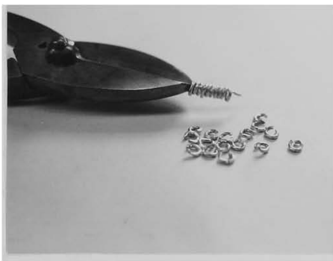
Fig. 2 Cutting the jump rings.
