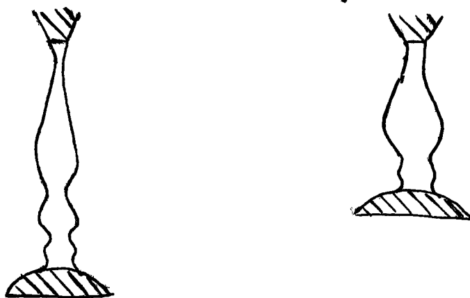
Fig. 3 Standing wave patterns on a liquid jet
