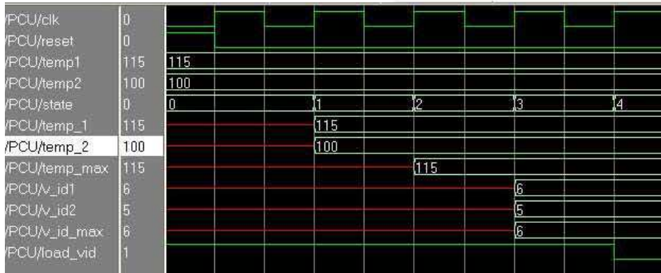
Figure 4.6: PCU Simulation Showing FSM State Flow.
