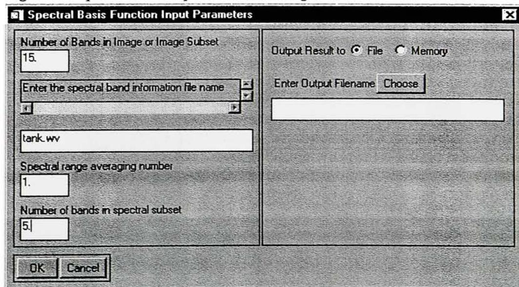
output in widget format as shown in Figure (19) where the user was able to click OK to continue with another iteration, or click CANCEL to end the routine and output final subset selection results to a widget.
