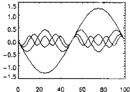
**Figure 4:** Summed Sine Curves - Step Function Approximation
