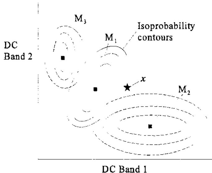
Each ellipsoid is representative of the GML discriminant value and centered about its multivariate mean  $\mathbf{M}$ . In this case, the pixel vector  $\mathbf{x}$  would be classified as a member of class 1. Diagonal ellipsoids are the result of correlation between class digital counts in the two spectral bands.
