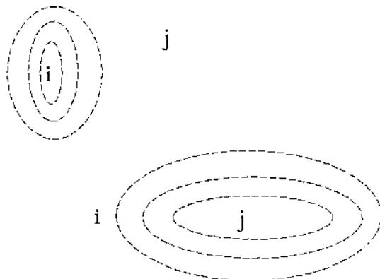
covariance matrix from class  $j$  is used. The dimensions of each ellipse in Figure (2) depend on the class variance from which the statistical distances are measured. Based on the ellipses shown, the variance for class  $i$  is considerably smaller than that of class  $j$ .
