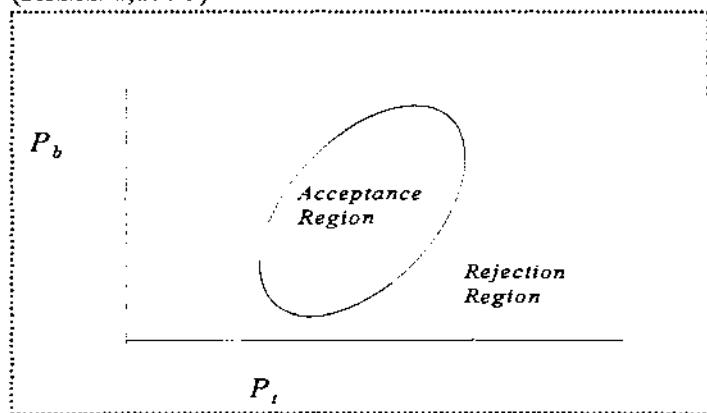
function, if  $l(\mathbf{x}) > P_t/P_b$ , the pixel is classified as target; if not, it is classified as background. A graphical representation of this classification process is provided in Figure (7).
