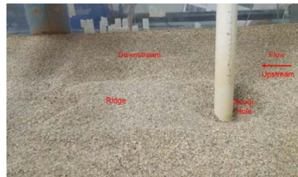
Fig. 4 Schematic of the scour hole and the ridge
