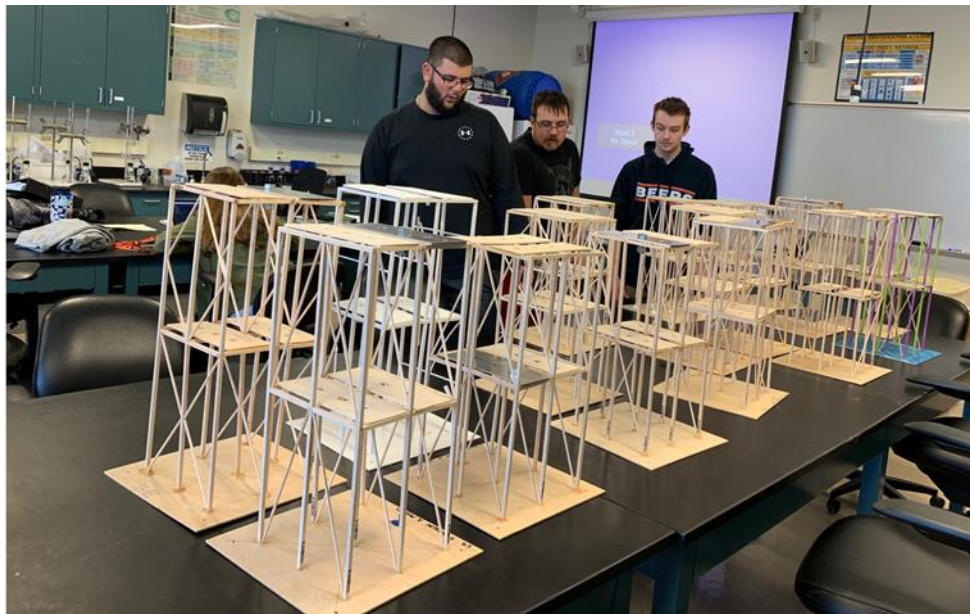
Figure 3: 2-Story Balsa Wood Models Built by Students
