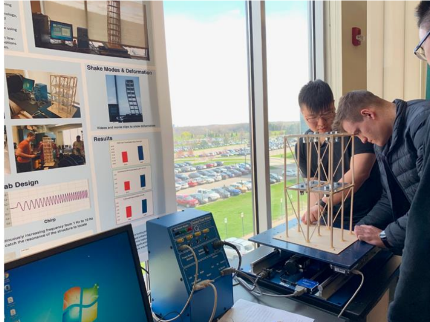
Figure 5: Students Mounting Building Model to Shake Table
