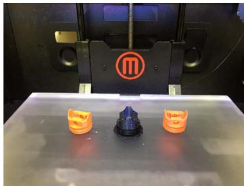
**Figure 1: 3D objects printed by material extrusion method**
