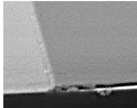
Figure 5: Zoomed-in view of oxide mandrel sidewall.
