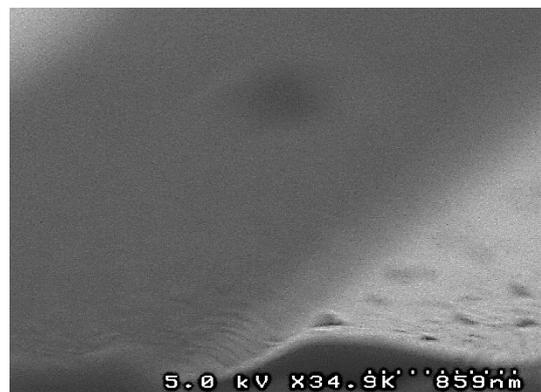
Figure 6: Oxide mandrel post silicon nitride etch.
