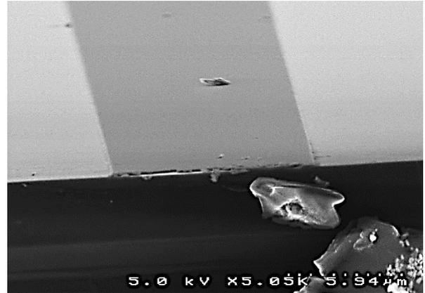
Figure 4: Wide oxide mandrel on silicon substrate.
