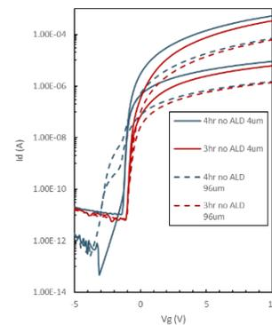
Figure 7: Anneal comparison of devices without an ALD capping layer
