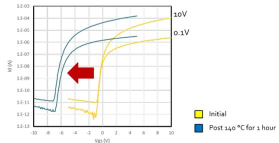
Figure 1: The voltage shift of a thermally stressed device
