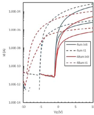
Figure 8: Length dependency of thermal stress
