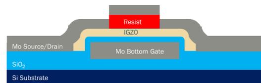
Figure 3: Cross section before metal lift-off for source/drain definition
