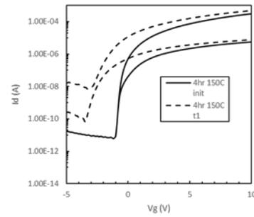
Figure 11: 4 hour anneal with 150 $^{\circ}\text{C}$  ALD
