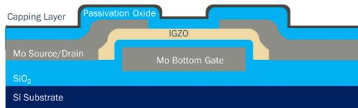
Figure 4: Cross section of device with added capping layer
