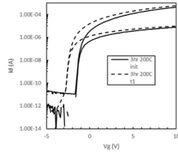
Figure 10: 3 hour anneal with 200 $^{\circ}\text{C}$  ALD
