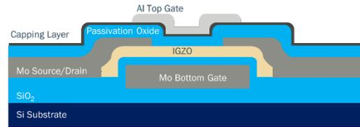
Figure 6: Completed device with capping layer
