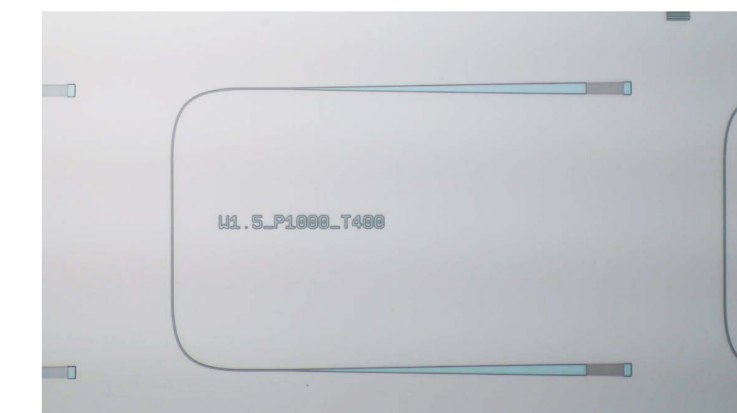
Fabricated Loopback Waveguide with 1.5µm width, 1µm coupler pitch, and 400µm coupler taper
