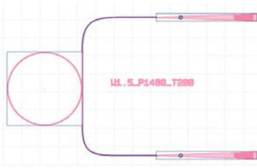
**Figure 2.** Shows Resonator Waveguide design for width of 1500nm and grating coupler pitch of 1400nm and 200nm taper.
