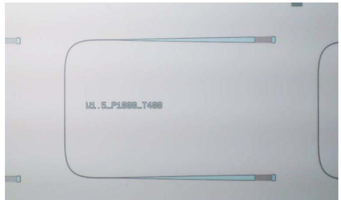
**Figure 14.** Shows fabricated loopback design with  $1.5\mu\text{m}$  wide waveguide and grating coupler pitch of  $1\mu\text{m}$  and  $400\mu\text{m}$  taper.
