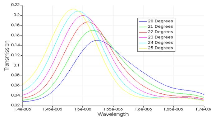
**Figure 18.** Shows simulation results for transmission versus wavelength when varying test head angle.
