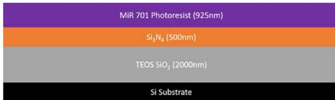
**Figure 7.** Shows wafer cross section following Photoresist coat.
