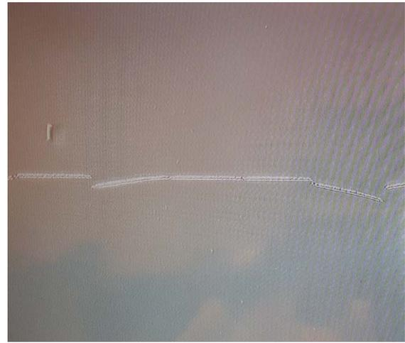
**Figure 13.** Shows photoresist adhesion problem with  $0.5\mu\text{m}$  lines.
