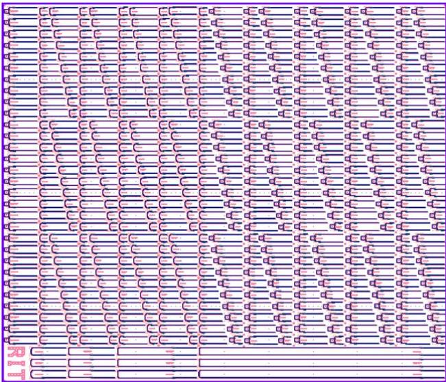
**Figure 3.** Shows mask design wave waveguide and grating coupler variations.
