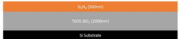
**Figure 6.** Show wafer cross section following LPCVD Nitride Deposition.
