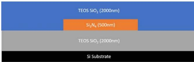
**Figure 11.** Shows wafer cross section following TEOS Cladding deposition.
