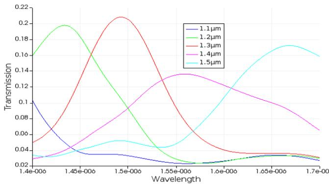
**Figure 19.** Shows simulation results for transmission versus wavelength when varying grating coupler pitch.
