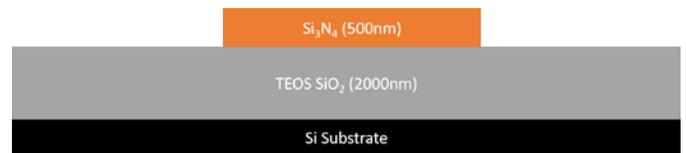
**Figure 10.** Shows wafer cross section following chemical photoresist strip.
