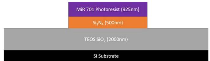
**Figure 9.** Shows wafer cross section following Nitride etch.
