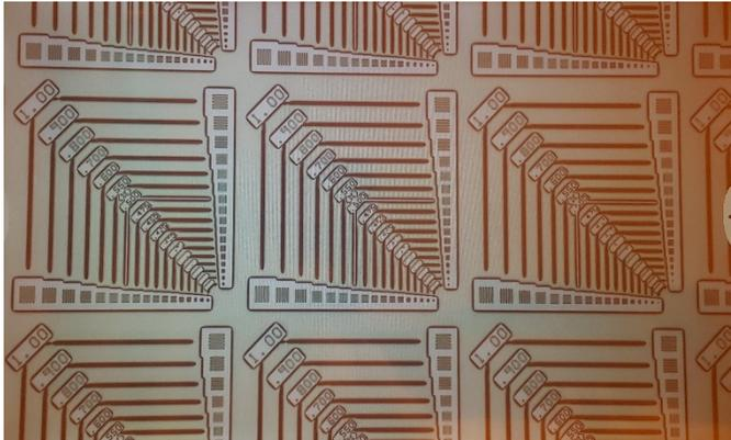
**Figure 12.** Shows Microscope capture of FEM to get correct exposure dose to resolve  $0.5\mu\text{m}$  lines.
