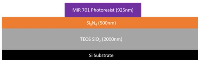
**Figure 8.** Shows wafer cross section following AMSL exposure and develop.
