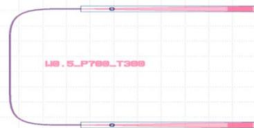
**Figure 1.** Shows Loopback Waveguide design for width of 500nm and grating coupler pitch of 700nm and 300nm taper.
