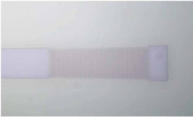
**Figure 15.** Shows microscope capture of grating coupler with 500nm lines and 500nm spaces.
