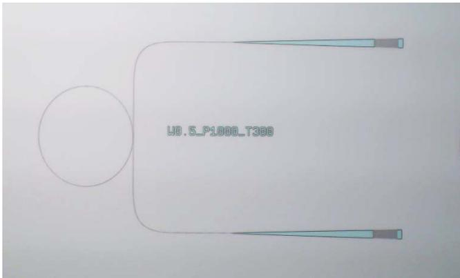
**Figure 16.** Shows fabricated ring resonator design with 0.5µm wide waveguide and grating coupler pitch of 1µm and 300µm taper.
