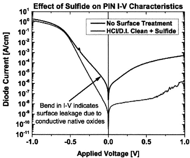
Fig. 5. I-V characteristics of a PIN diode treated with and without the HCl/D.I. H<sub>2</sub>O clean.
