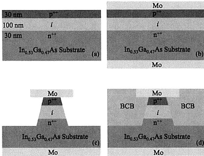
Fig. 2. (a) Starting Substrate. (b) Top side and back side Mo contact deposition. (c) Mo dry etch (SF<sub>6</sub>) and InGaAs citric acid wet etch. (d) Surface clean, sulfide passivation, BCB application, cure and etch back.
