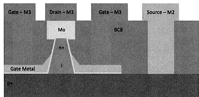
Fig. 1. Cross section of a basic III-V based mesa structured Tunneling FET.
