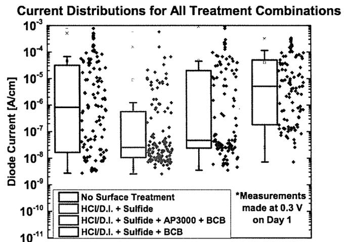
Fig. 3. *I*<sub>0</sub> distributions in Amperes per unit perimeter length for each analyzed treatment combination.
