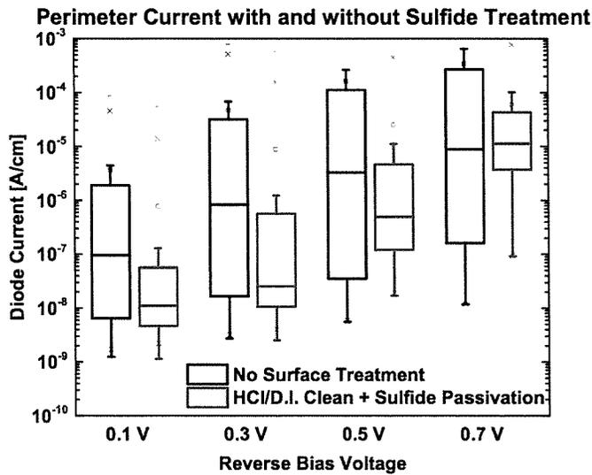
Fig. 4. Comparison of devices with and without HCl/D.I. H<sub>2</sub>O Clean & Sulfide Passivation.
