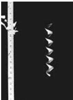
SPINNING SEED IS PHOTOGRAPHED WHILE FALLING NEXT TO A YARDSTICK WITH THE CAMERA SHUTTER SET TO 1/4 SECOND. IN THAT TIME THE SEED FALLS 11 INCHES FOR AN AVERAGE VELOCITY OF 44 INCHES PER SECOND. IN THE SAME TIME IT TURNS ABOUT 5.5 TIMES FOR A ROTATION RATE OF 22 RPS OR 1320 RPM
