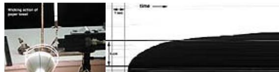
The image obtained clearly shows the significant change in velocity of the dye as it rises ever higher along the length of the hanging, absorbent, paper. At first there is significant acceleration of the ink upwards. With time, however, the rate of ascent slows down and eventually, in fact, it stops altogether as all the dye becomes absorbed by the paper or when evaporation plays a significant role in the dye transport process.
