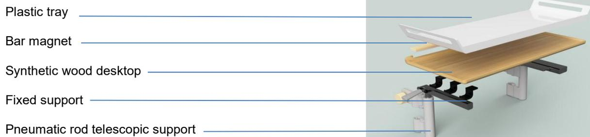
Figure 10. Structural explosion diagram
