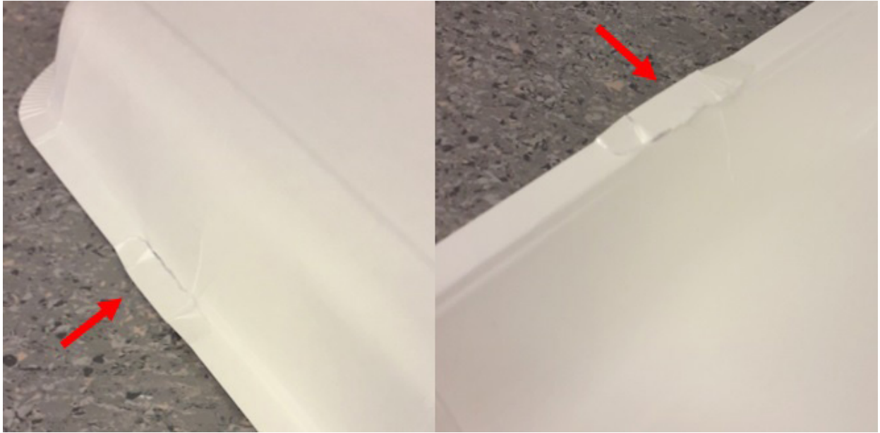
Fig. 11: Detected breaks in a tensile tested tray observed from bottom (left) and top (right) of the tray, the breaks are highlighted with arrows.
