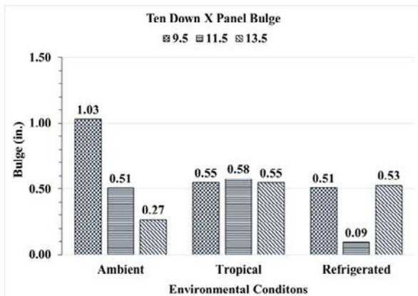
Fig. 19: 10-Down RSC's Compression Bulge Displacement along X Panel (Long Face)
