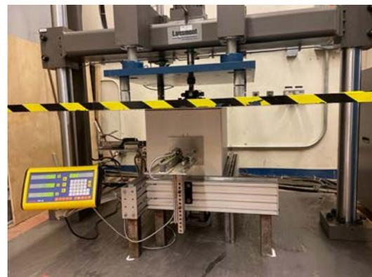
Fig. 16: Compression Bulge Displacement Test Set-Up
