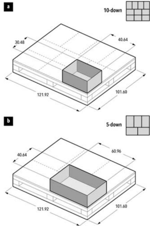
Fig. 5: (a) Half-size (b) Full-size Corrugated Common Footprint (CCF) Containers [12]
