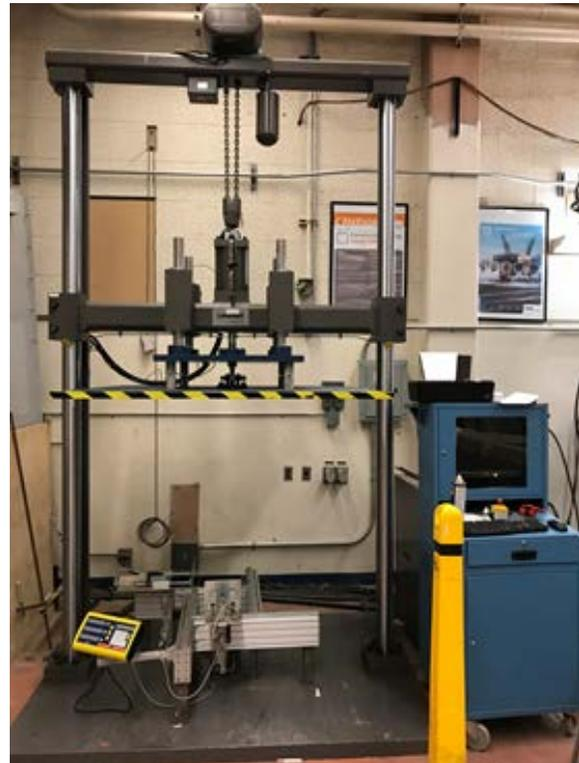
Fig. 13: Bulge Measuring Apparatus and Lansmont Compression Tester
