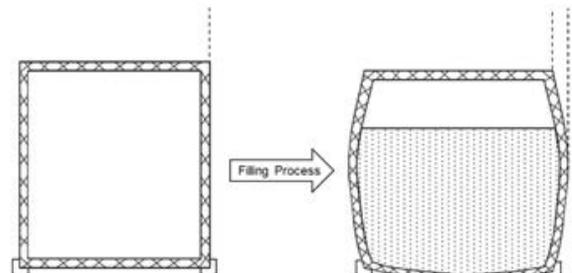
*Fig. 7: Initial Bulge of a Container During Filling Process [12]*
