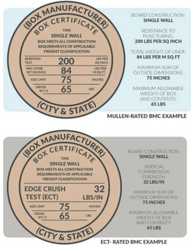
Fig. 2: Mullen and ECT-rated Box Manufacturer Certificates [8]
