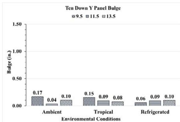
Fig. 20: 10-Down RSC's Compression Bulge Displacement along Y Panel (Short Face)
