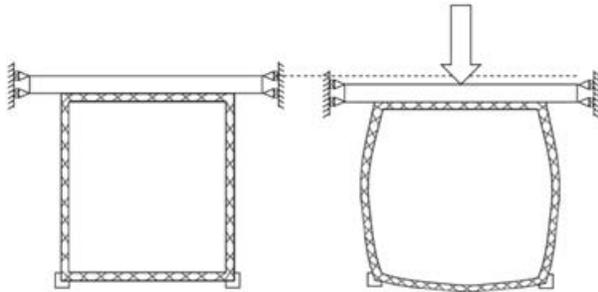
*Fig. 6: Container Bulge of an Empty Container Under Compression [13]*
