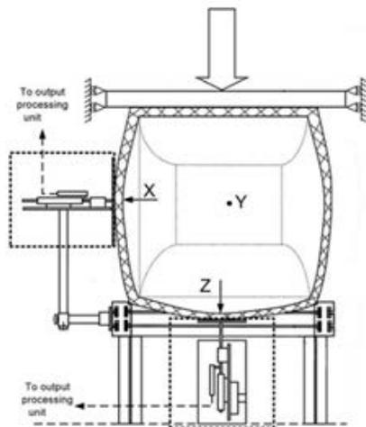
Fig. 12: Cross Sectional View of a Container During Compression Bulge Test
