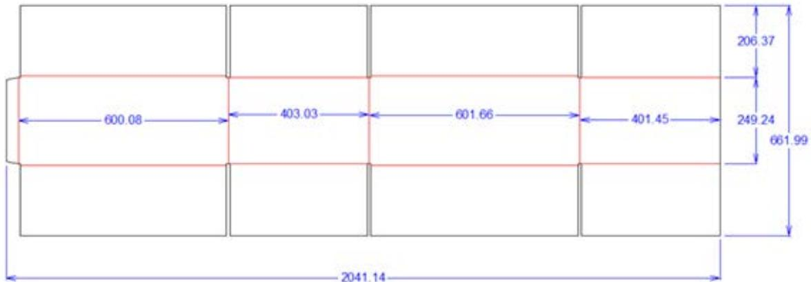
Fig. 9: Ten-Down Box Design Example – 9.5-inch height (241.3 mm) [All dimensions are in millimeters]
