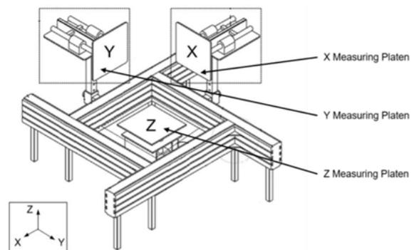
Fig. 11: Perspective View of the Bulge Measuring Apparatus [Adapted from US Patent US8746085B2] [17]
