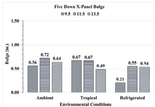
Fig. 17: 5-Down RSC's Compression Bulge Displacement along X Panel (Long face)
