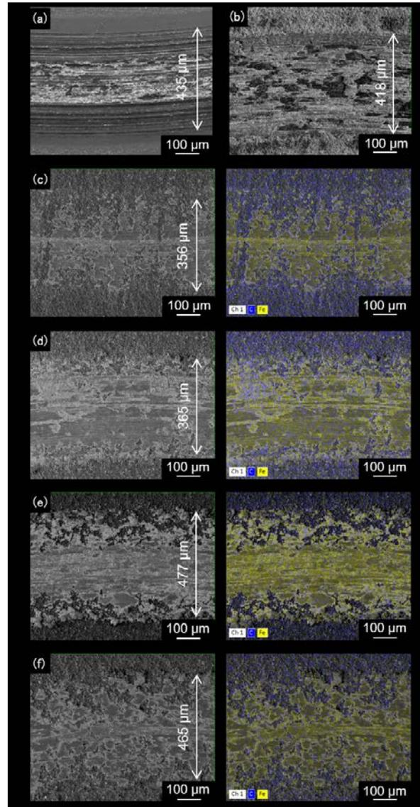
Figure 8. SEM images and EDX maps of wear tracks after ball-on-disk tests. a) Control substrate. b) Substrate with  $R_a=1.0\ \mu\text{m}$ . AP-DLC coatings on substrates with various  $R_a$ s: c)  $0.9\ \mu\text{m}$ , d)  $1.0\ \mu\text{m}$ , e)  $1.3\ \mu\text{m}$ , and f)  $1.4\ \mu\text{m}$ . C (blue) and Fe (yellow) in the wear tracks are shown in the EDX maps.
