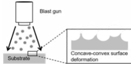
Fig. 1: Schematic diagram of the FPB process.
