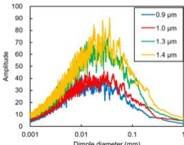
Fig. 6: Distribution of dimple diameters on substrates with various surface roughness.
