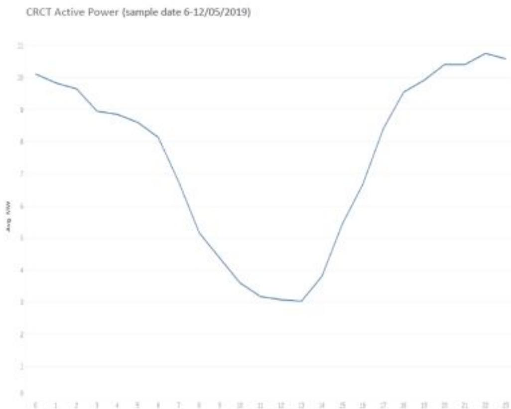
Figure 15: Load Profile of CRCT (P, MW)
