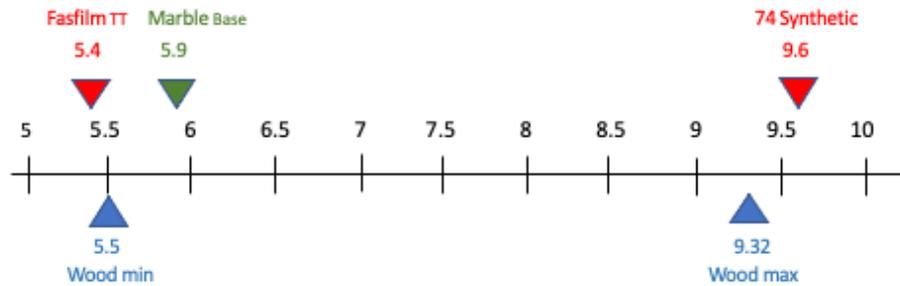
Figure 19. Tensile Strength (MD) for Synthetic and Stone v. Wood
