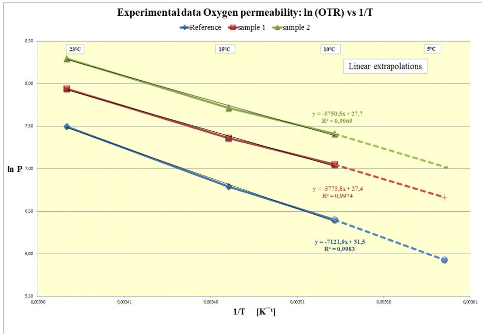
Figure 2 showed OTR experimental data with trend line and R square values compared to standard BOPP of films containing EOC in the core.
