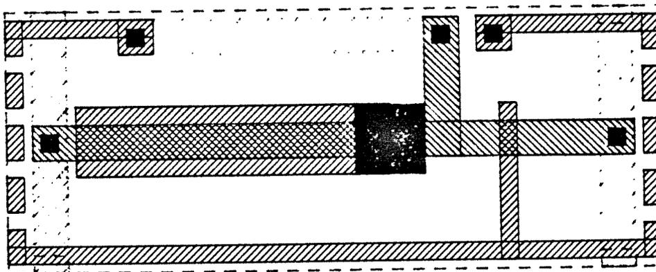
Figure 4: Design of Inverter Standard Cell in CHIPGRAPH
