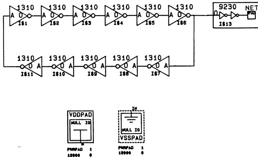
Figure 2: Schematic of Ring Oscillator in NETED
