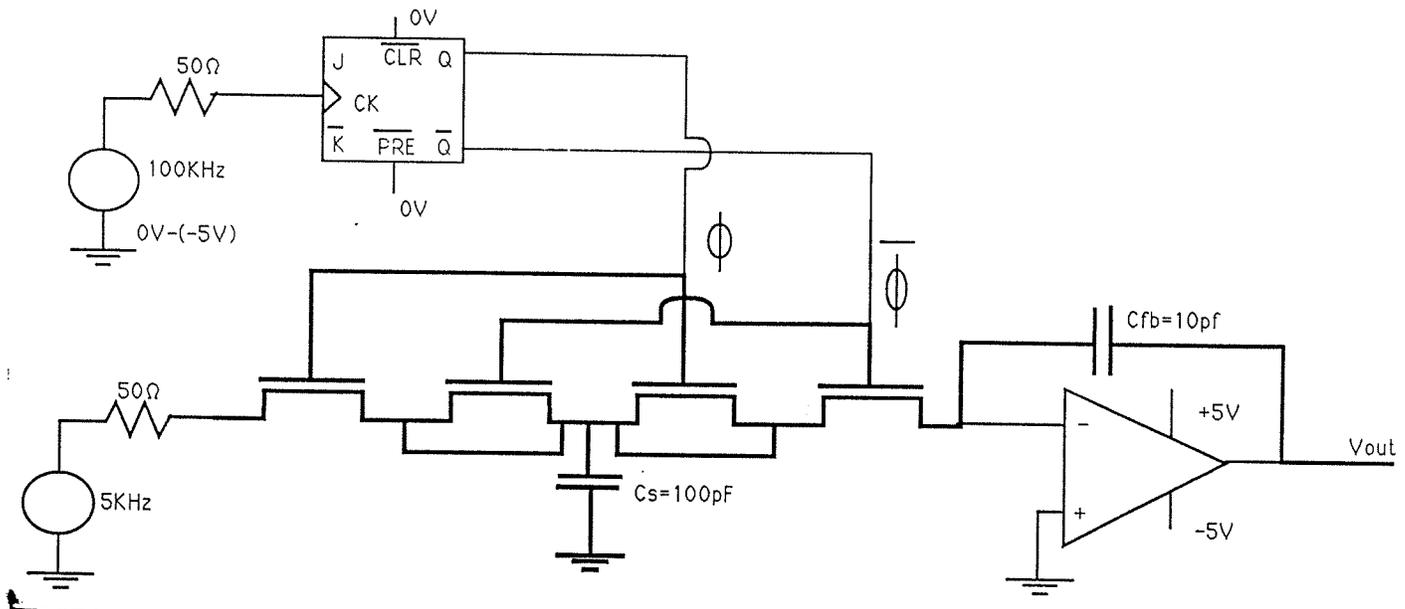
Figure 2b: Design Schematic of Integrator Op Amp
