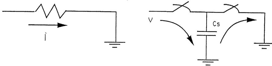
FIGURE 2a: THE SWITCHES ON THE RIGHT WILL SERVE THE SAME PURPOSE AS THE RESISTOR ON THE LEFT.
