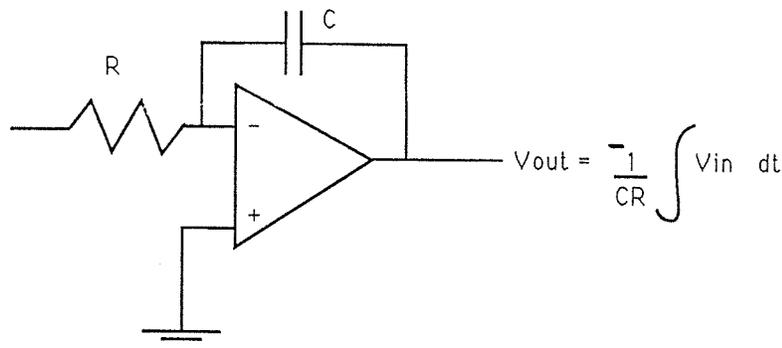
FIGURE 1: SCHEMATIC OF INTEGRATOR CIRCUIT
