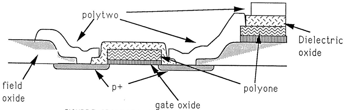
FIGURE 3: CROSS SECTION OF SELF ALIGNED DOUBLBLE POLY PROCESS
