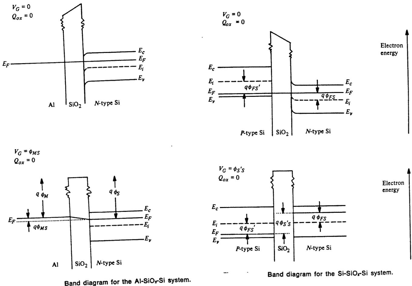
When the aluminum gate is replaced by the doped polysilicon gate, the work function between the gate electrode and the silicon substrate is changed. By assuming that a band analysis is valid for the polycrystalline silicon, the effective work function difference ( $\phi_{igs}$ ) is given by the equation
