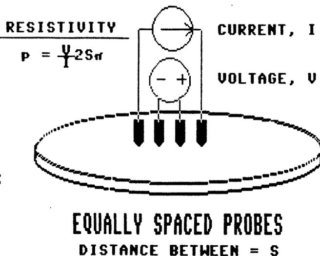
Figure 1: Four Point Probe
