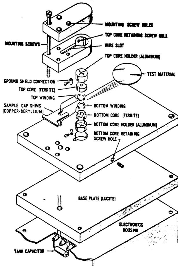
Figure 5: Header Assembly [1]
