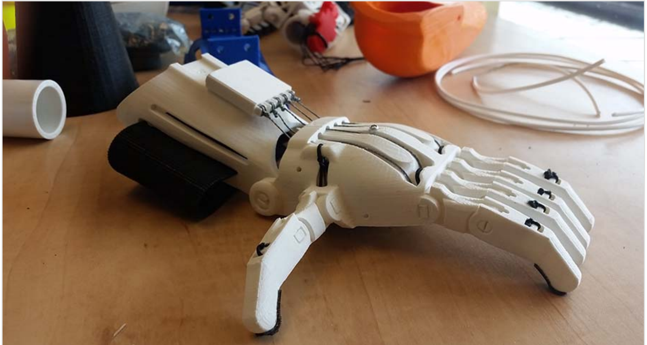
Figure 1. A 3D-printed upper-limb assistive technology device (e-NABLE Raptor Reloaded hand design). Photo: Jeremiah Parry-Hill. November 12, 2015.
