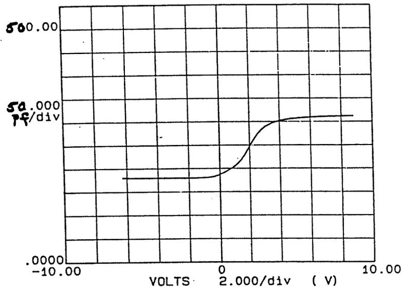
Figure 2: Capacitance vs. Voltage ( $4 \times 10^{12}/\text{cm}^2$  dose, no sinter)
