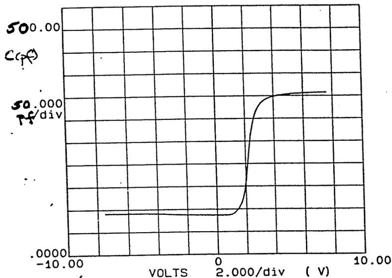
Figure 1: Capacitance vs. Voltage (no implant or sintering)
