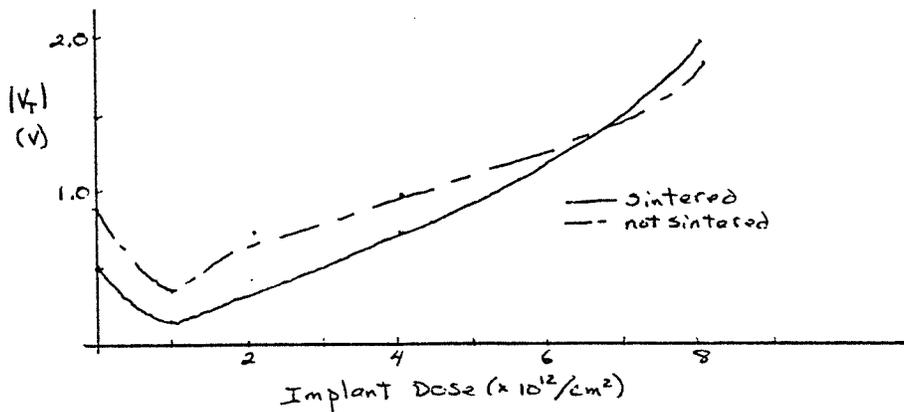
Figure 3: Threshold Voltage Magnitude vs. Implant Dose
