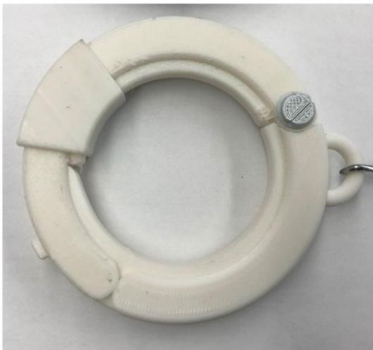
Figure 4. Early Iteration of Cuff with Stop for Cap
