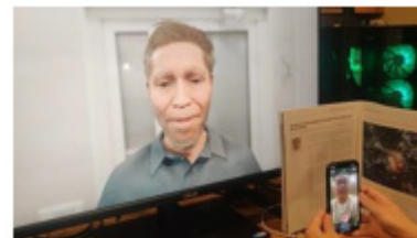
Fig. 2. Live Link Face real-time facial/eye movements transmitted from iPhone to PC/Unreal software to then transfer, in real-time, to mannequin iPad
