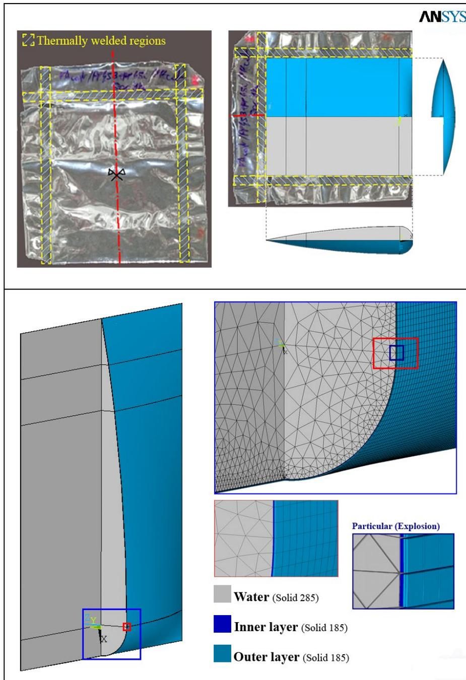
Fig. 2. Typical food package polymeric bi-layer structure and three-dimensional model used in the FE simulations. Geometry and details of the mesh for the food package Finite Element model
