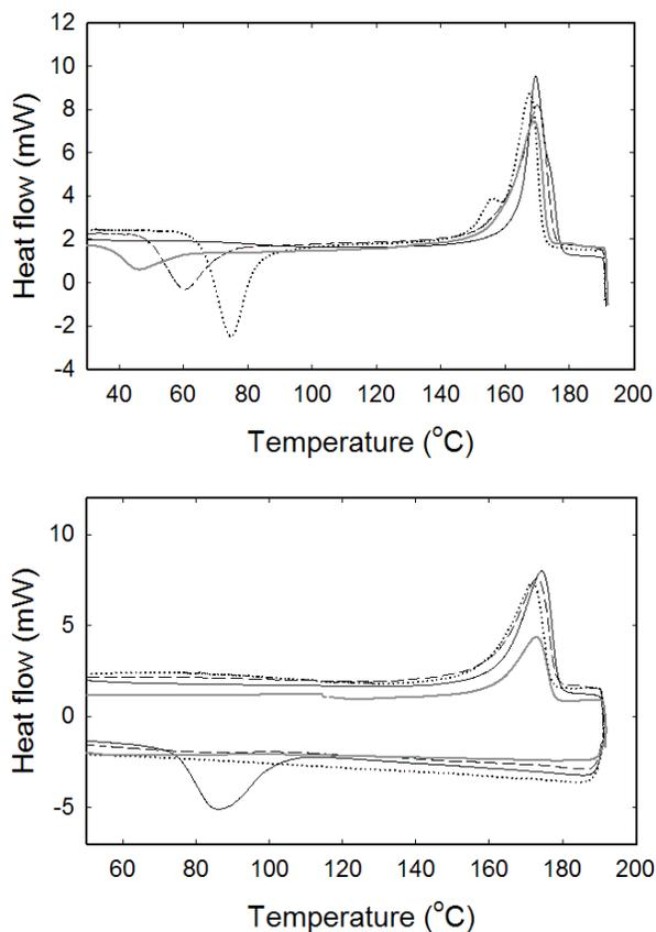
Fig. 2. DSC of neat PHB (solid line), of the PHB/TA10 (broken line) compounds
