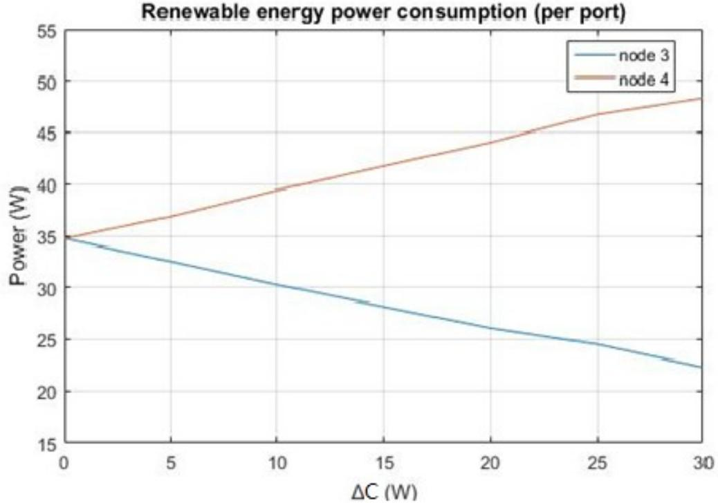
**Figure 4.4:** Renewable Energy Power Consumption between node R3 and R4 (per port)
