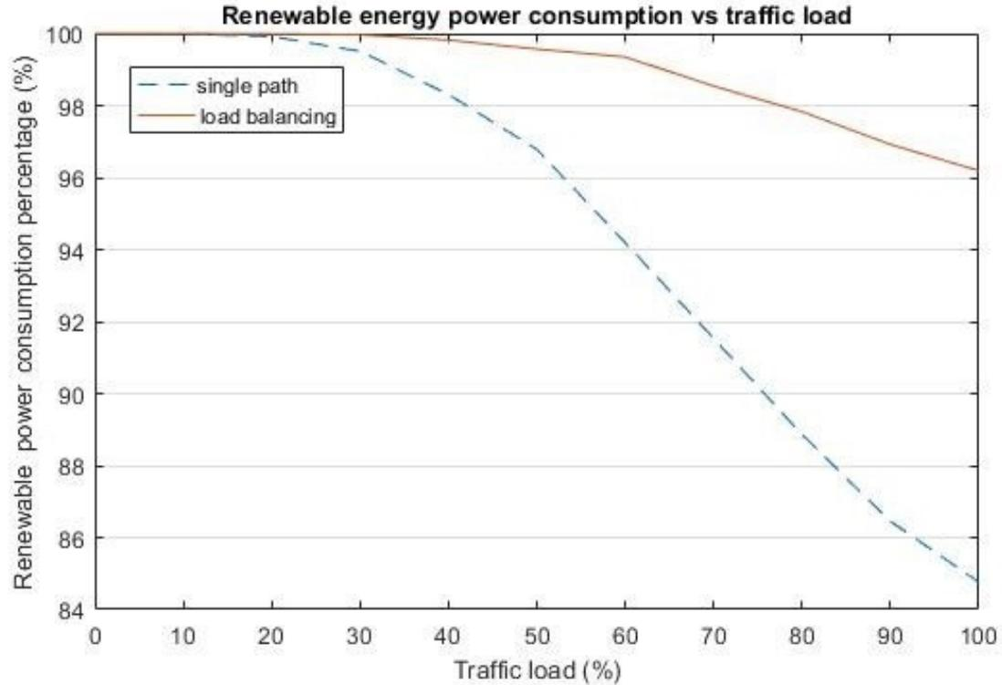
**Figure 5.3:** Renewable energy power consumption vs traffic load with scenario 1
