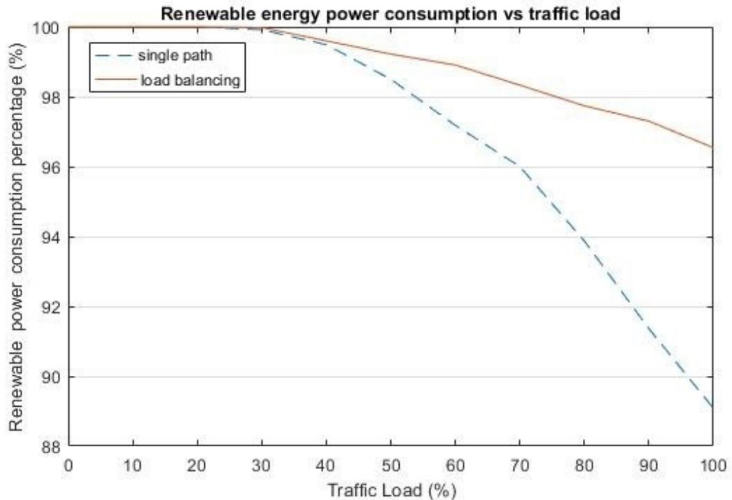
**Figure 5.5:** Renewable energy power consumption vs traffic load with scenario 2
