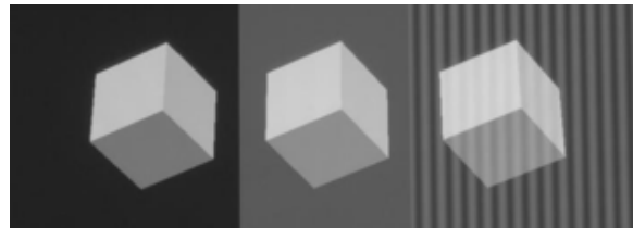
Fig. 1 Photograph of three identical cubes rendered in an OST AR against different backgrounds: dark-solid, light-solid, light-patterned (from left to right).
