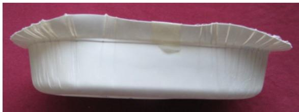
*Figure 7. A deformed tray due to a high temperature (160 °C).*
