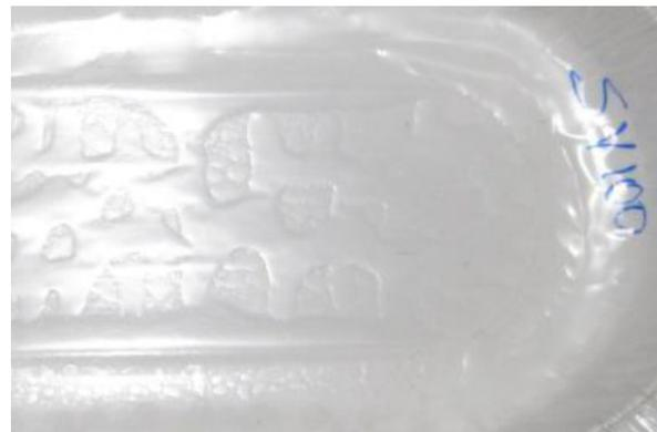
Figure 5. Air bubble formation in a press formed tray, coated with Multifol SV 100 film.
