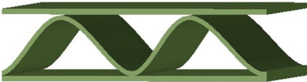
Figure 5: Approximate sine wave shape of the corrugated paperboard fluting used in the finite element model of the edge compression test
