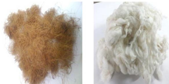
*Figure 1: Treated coir (left) and cotton fiber (right)*
