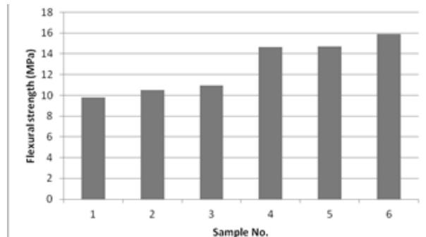
Figure 4: Flexural strength comparison of different composite material
