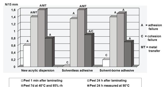
In figure 5 it is also demonstrated that with regard to green strength the aqueous adhesive is also superior to the solvent-borne adhesive, though not to such a high degree as to the solventless system. This is due to the higher molecular weight of the solvent-borne system (figure 4). Because of their high green strength, inline converting processes such as an inline slitting of the laminate roll becomes possible for converters who use water-based adhesives.
