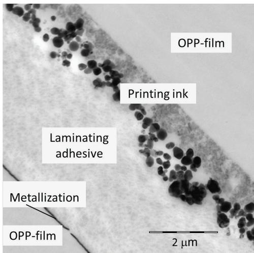
In figure 3 a reverse printed OPP film has been dry laminated to a metallized OPP film, which had been coated with a new developed aqueous acrylic dispersion as a laminating adhesive. A good wetting onto the rough colour pigment surface is visible here resulting in high bond strengths of the laminate. Another consequence of the good wetting is an excellent brilliance of the print.
