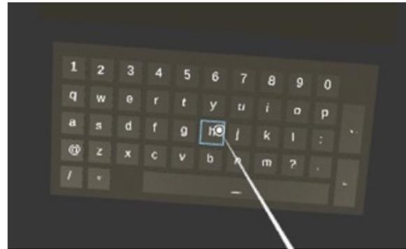
*Fig. 5. Raycasting: moving the controller in space and casting the virtual ray to a particular key to highlight it*
