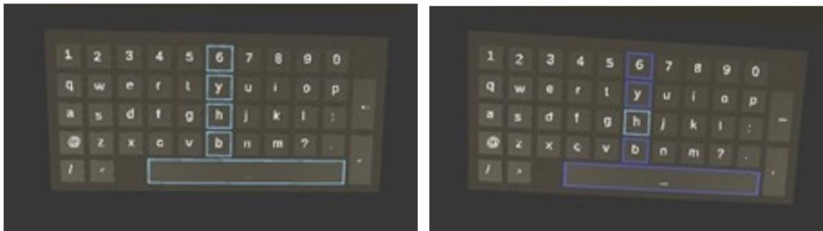
Fig. 4. RCR: (left) rolling the controller to switch the highlighted column (light blue outline), press the trigger button on the controller to lock the highlighted column; (right) Once a column is locked, rolling the controller to move the cursor (light blue outline) up and down within the locked column (dark blue outline)
