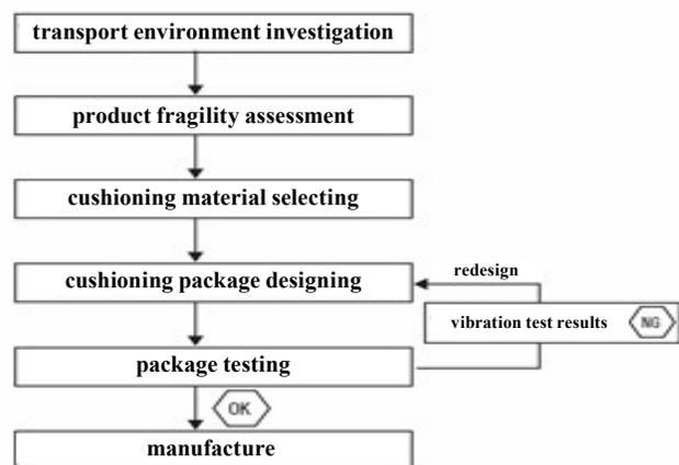
Figure 1: A simplified flowchart of the traditional cushioning package design.
