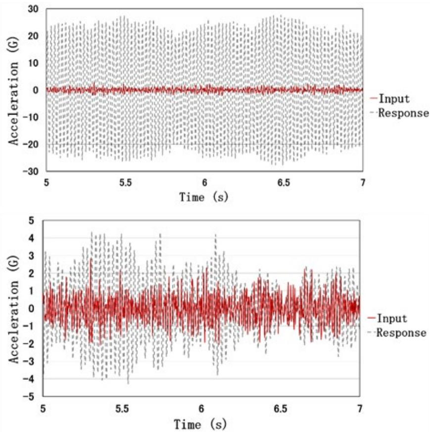
Fig.10 The vibration input and vibration response of type (a): (a) 1% Strain and (b) 5% Strain.
