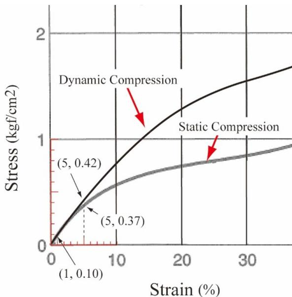
Fig.9. The Dynamic and Static Stress–Strain curve of Eperan™ XL38.
