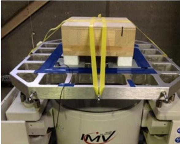
Fig.11 Vibration transmissibility test.
