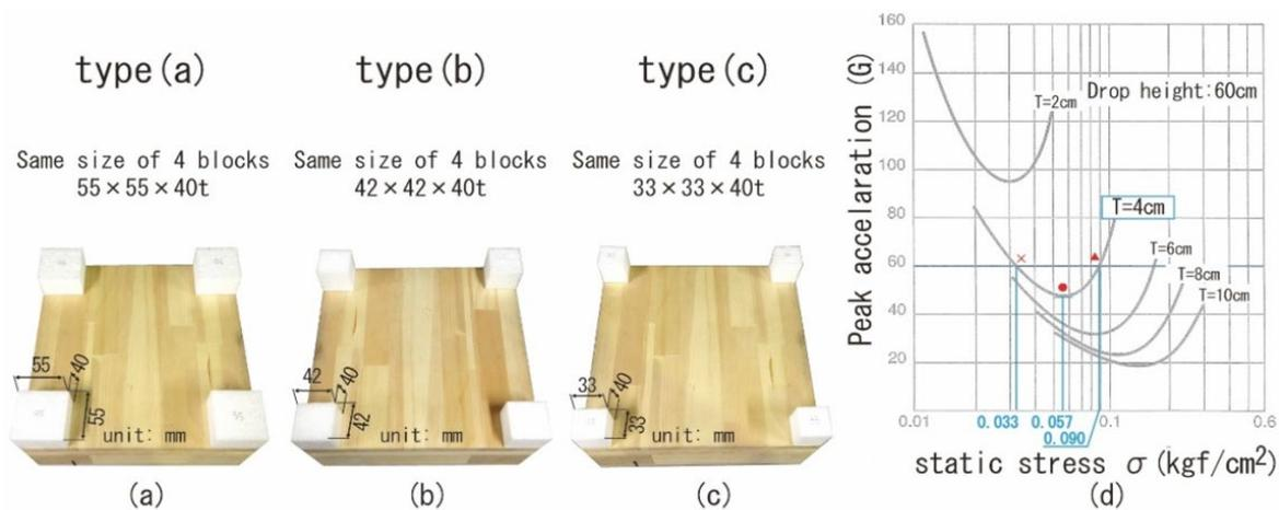
Fig.8 Cushion curve and dummies based on selected stresses. (a)  $\sigma_s=0.033 \text{ kgf/cm}^2$ , (b)  $\sigma_s=0.057 \text{ kgf/cm}^2$ , (c)  $\sigma_s=0.090 \text{ kgf/cm}^2$  and (d) cushion curve of Eperan™ XL38.
