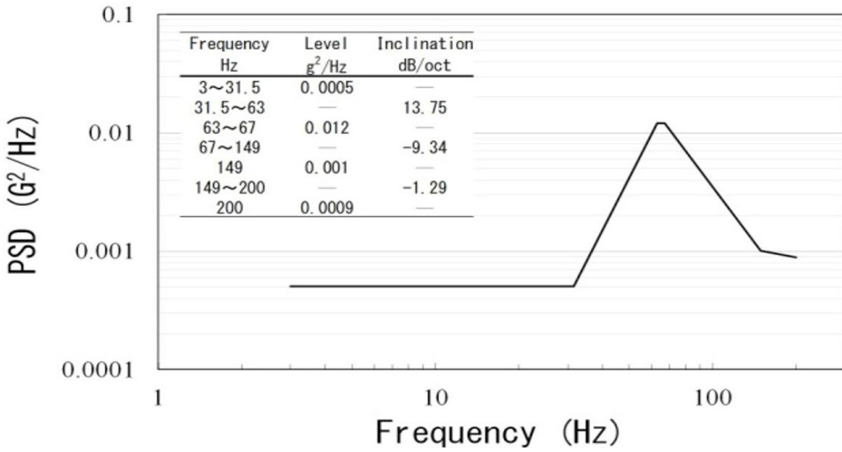
Fig.6: PSD of assumed transport environment
