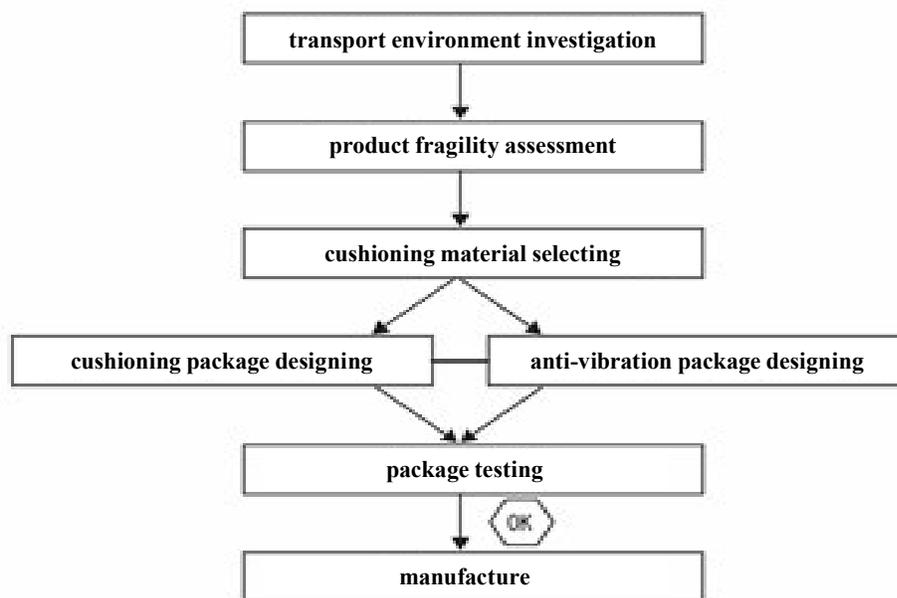
*Fig. 2: The simplified flowchart of the Hybrid Damping Package Design<sup>6</sup>.*
