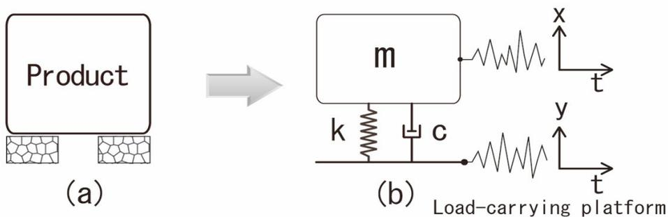
Fig.4 The viscous damp model (VD model): (a) Cushioned Package and (b) VD model.
