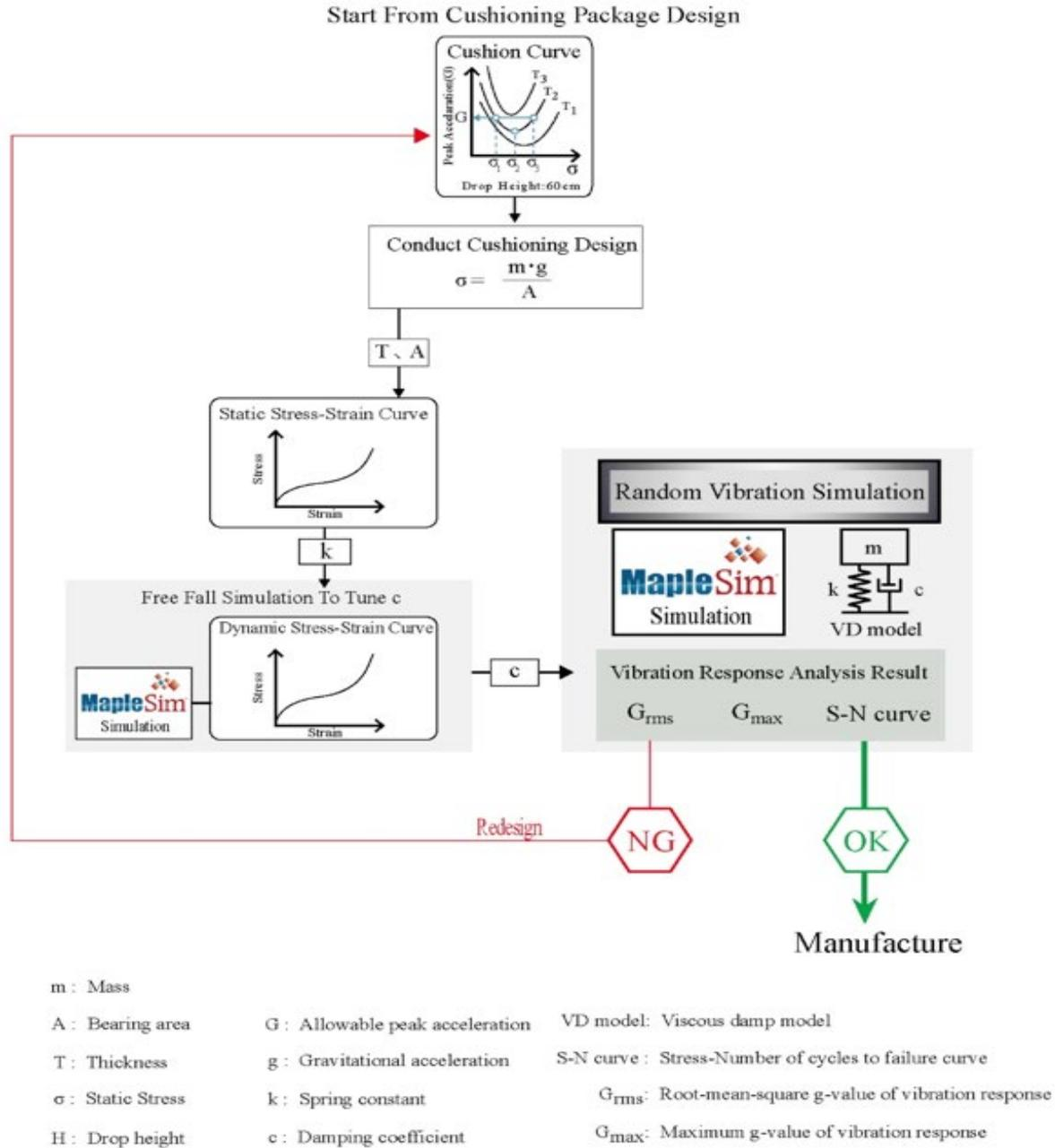
Fig.5. The flowchart of the Hybrid Damping Package Design process.
